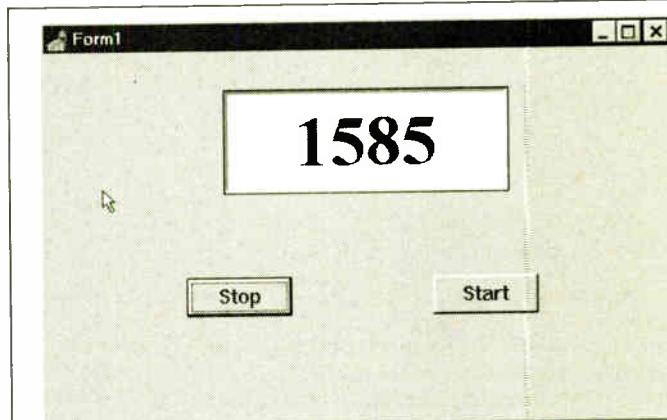
Fig.4. The converter program in action. The maximum reading is 4095.
