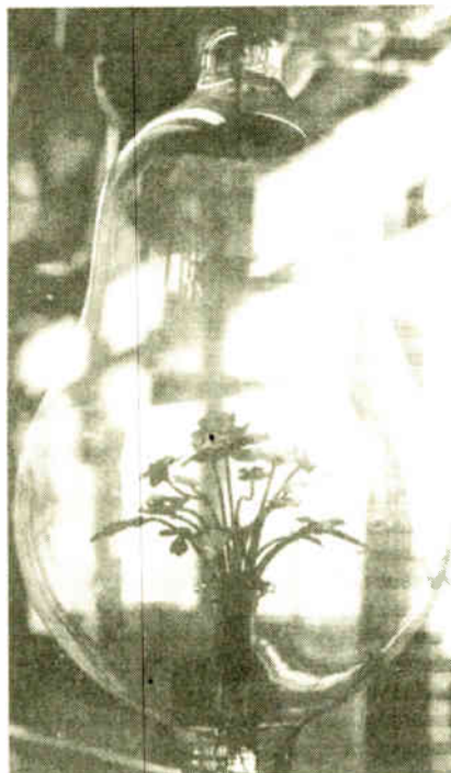
An early ornamental Crookes' tube, with metal flowers which glowed when a current flowed.
