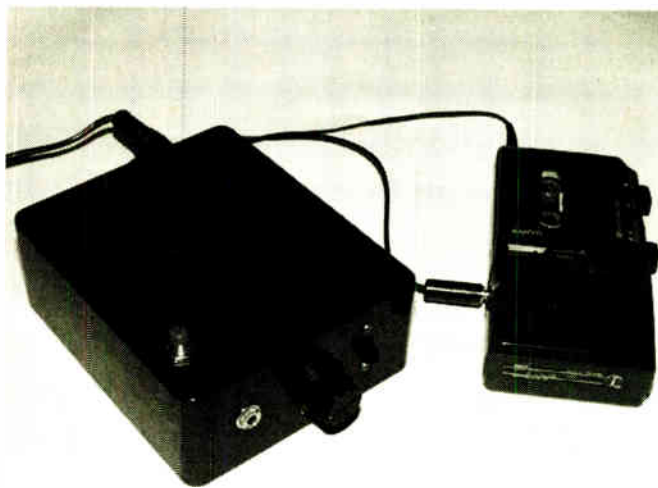
Completed Easy-Typist showing additional pause switch button on top of the case.
