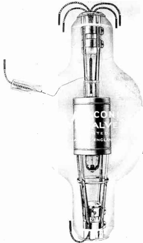
Fig. 4.—A WIRELESS VALVE IN WHICH PURE NICKEL IS USED FOR THE GRID, GRID SUPPORTS, PLATE, ETC. (The Marconi Co., Ltd.)
