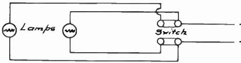
Fig. 2A.—WIRING CONNECTIONS FOR SERIES-PARALLEL CONTROL OF TWO FITTINGS. Lamps in parallel for full light.
