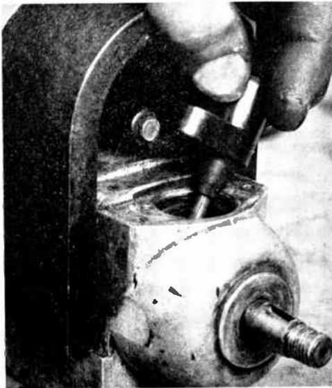
Fig. 4. —ANOTHER STEP IN DISMANTLING A MOTOR CAR MAGNETO.
