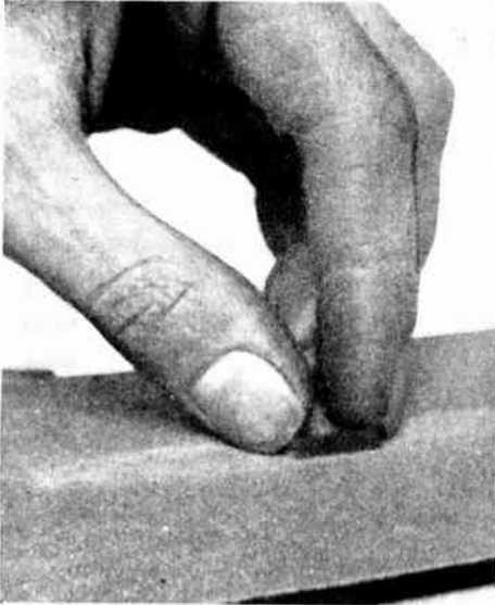
Fig. 16.—REMOVING THE BURRS FROM THE COPPER SEGMENTS BEFORE THEY ARE ASSEMBLED FOR TURNING.
