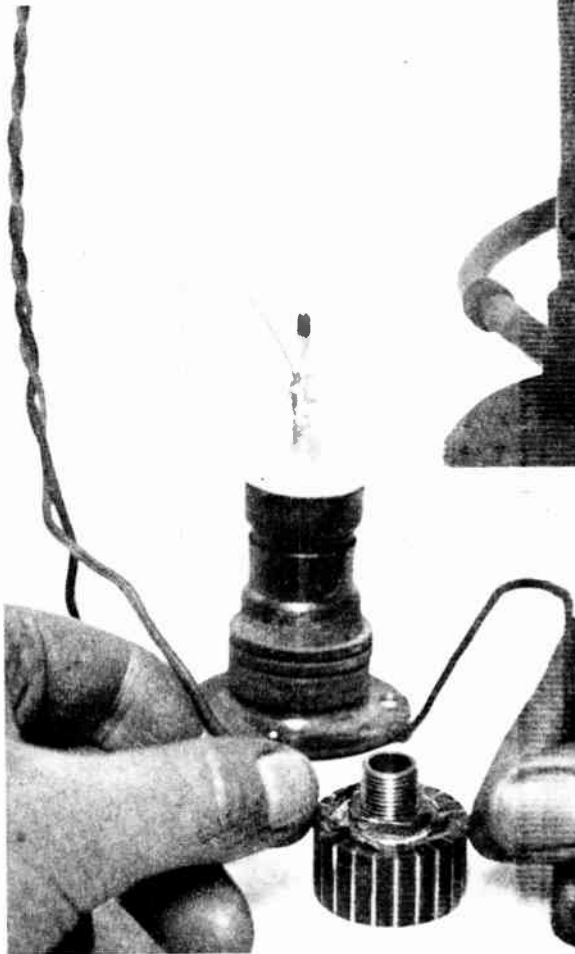
Fig. 23 (Left). TESTING THE INSULATION OF THE COMMUTATOR AFTER REMOVING IT FROM THE CLAMP.
