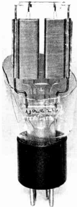
Fig. 6.—THE CONSTRUCTION OF A "MULLARD" FULL-WAVE RECTIFIER VALVE.
