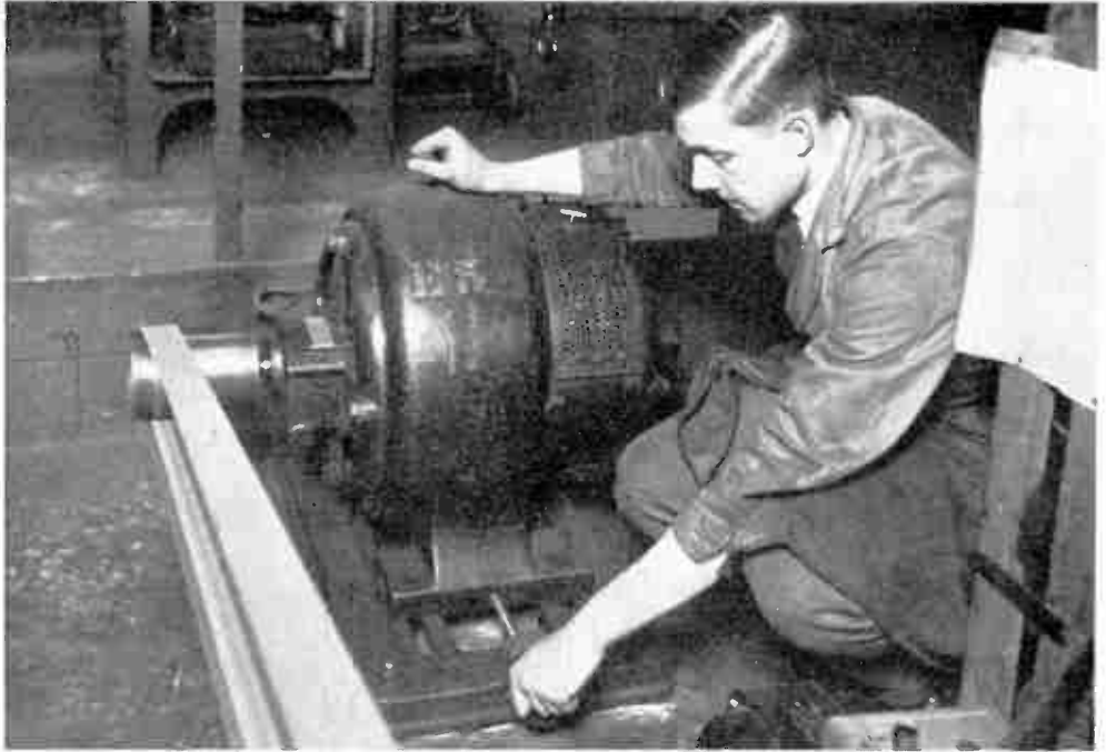
Fig. 3.—TIGHTENING THE BELT OF A MOTOR BY MOVING THE MACHINE ON THE RAIL. ( Lancashire Dynamo and Crypto Ltd. )
