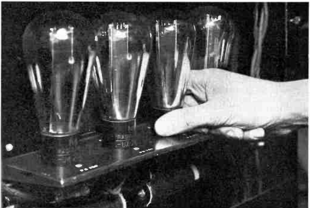
Fig. 41. —CORRECT METHOD OF REMOVING A VALVE.
