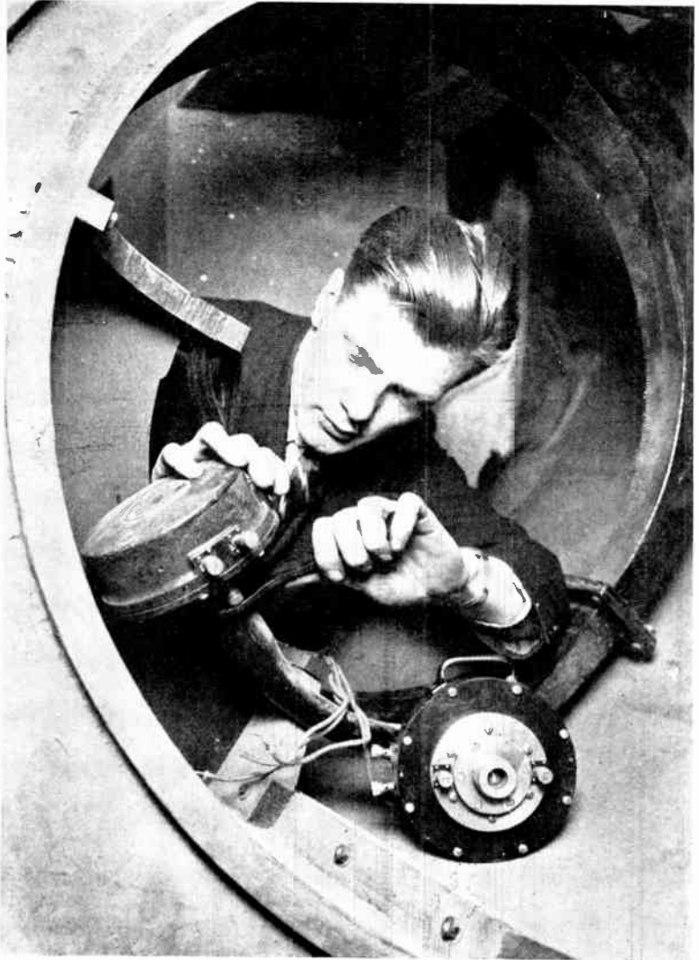
Fig. 19. —How THE RECEIVER IS CONNECTED TO THE HORN.
