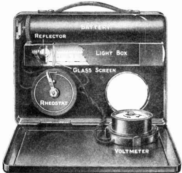
Fig. 11.—EDISON SWAN PORTABLE PHOTOMETER.
