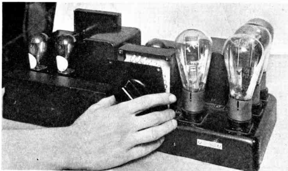
Fig. 38. —REMOVING THE VOLUME CONTROL FROM THE TYPE PG-13 AMPLIFIER.
