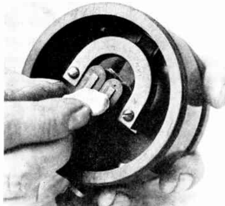
Fig. 3.—CLEANING THE TIPS OF THE POLES.
