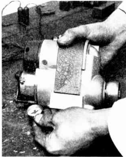
Fig. 1.—TESTING POLARITY OF A MAGNETO.
