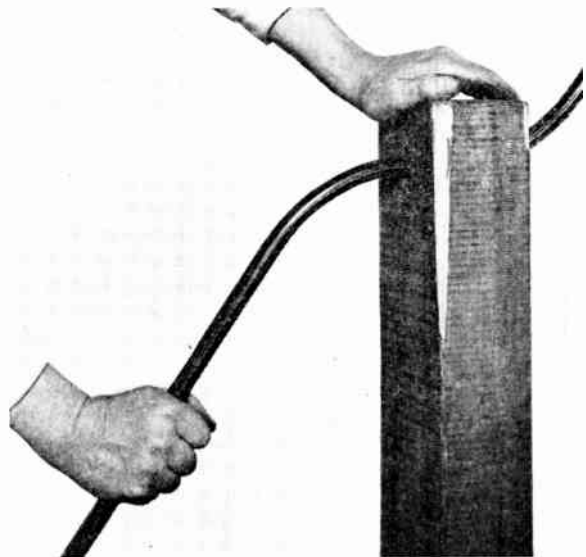
Fig. 4.—MAKING A "SET-OFF" ON A PIECE OF CONDUIT.
