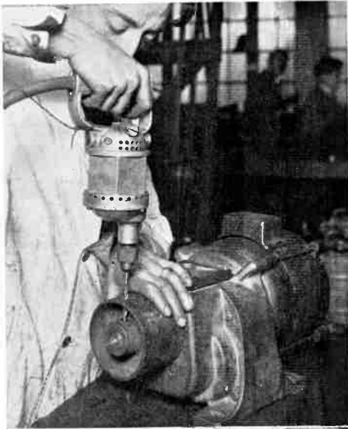
Fig. 50B (Right). FITTING THE DRIVING PULLEY TO A GEARED MOTOR.
