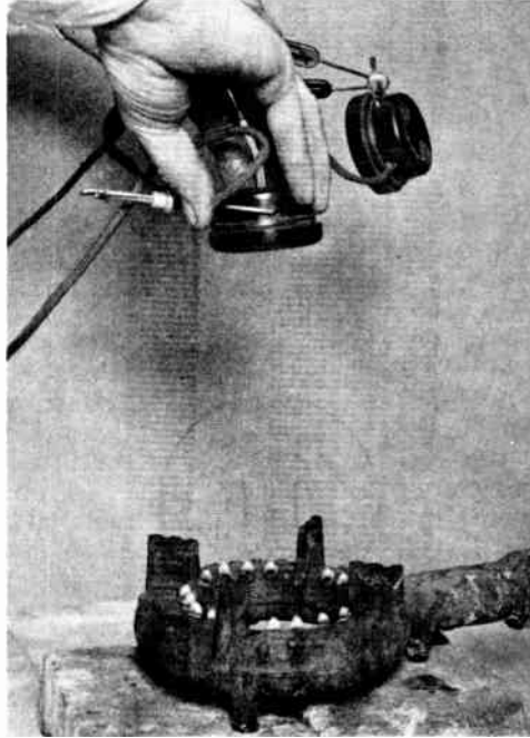
Fig. 1.—HOW TO LOOSEN A TIGHT EARPIECE.
