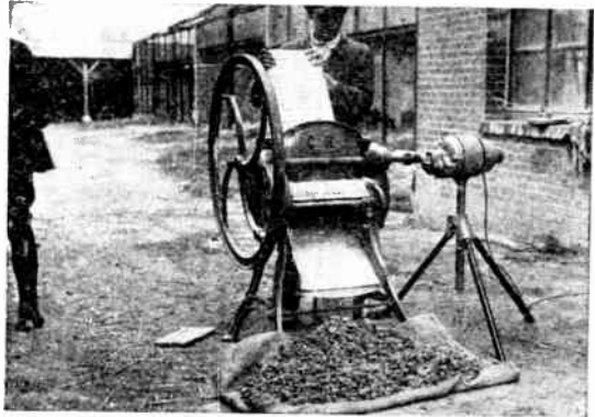
Fig. 51.—PORTABLE MOTOR DRIVING A CATTLE CAKE - BREAKING MACHINE. (J. Harrison & Co., Ltd.)
