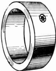
Fig. 13.—COLLAR FOR LOCATING SHAFT. Note setscrew to grip shaft.
