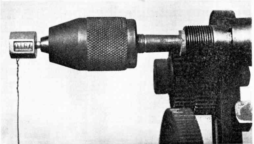
Fig. 5. —A SIMPLE METHOD OF MOUNTING A COUNTER ON THE LATHE.
