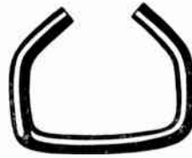
Fig. 35B.—ROUND WIRE FASTENERS. The wire is put through a hole in end of belt and clinched over.
