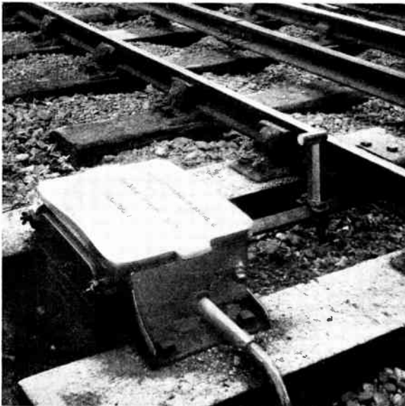
Fig. 5.—THE LONDON ELECTRIC RAILWAY ELECTRICALLY SIGNAL-OPERATED TRAIN STOP AS SUPPLIED TO THE METROPOLITAN RAILWAY; WESTINGHOUSE PATTERN.
