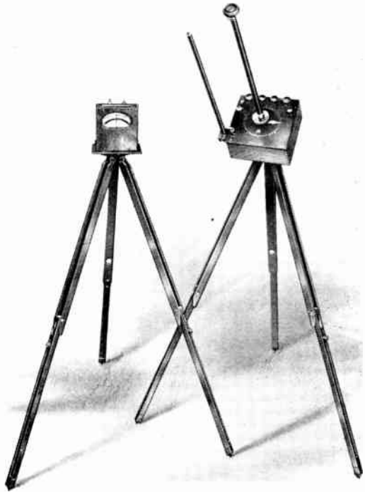
Fig. 8.—HIGHLY INSULATED SLIDE WIRE BRIDGE AND GALVANOMETER.
