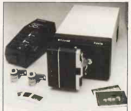
The Polaroid Palette shoots an image straight on to 35mm. film.
