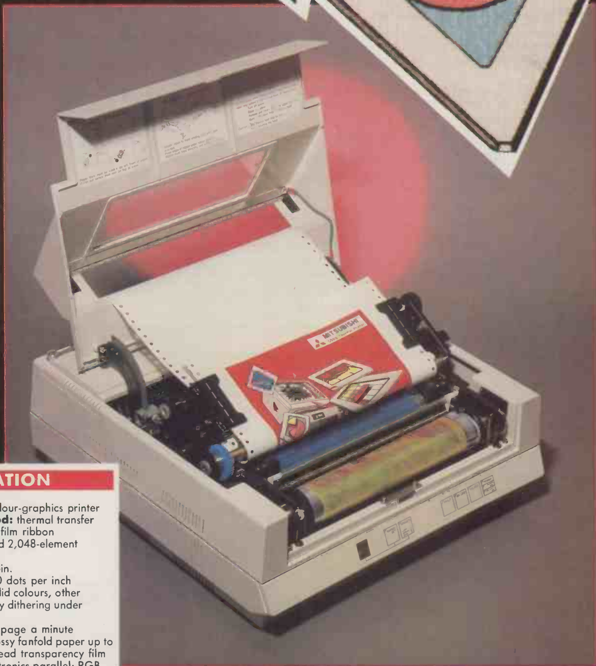
The G-500 opened up to show the three-colour film roll at the front.
