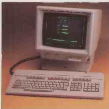
There is a choice of intelligent text-only terminals (above) or bit-mapped colour units (right) to run Gem software.
