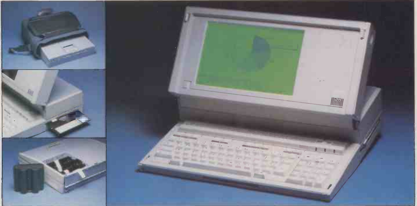
Two plus points of the Olivetti M-22 are its clear back-lit LCD screen and its ability to use a hard disc.
