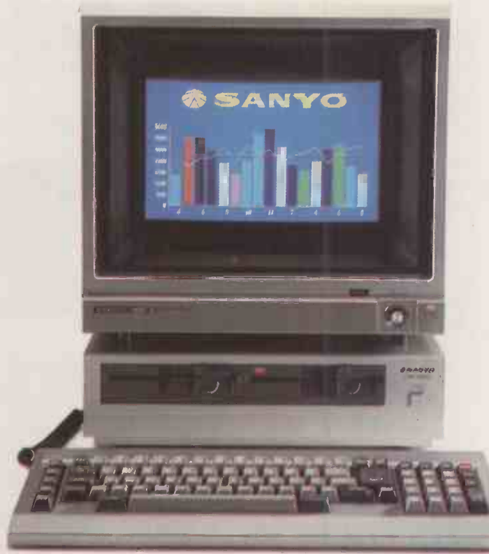
MBC 555-2 £1,190 + VAT.* MS-DOS 2.11. 128K RAM expandable to 256K. 2 x 360K drives. RGB colour/mono outputs. Centronics compatible printer port. Audio training tape. Free Wordstar, Calcstar, Mailmerge, Spellstar, Reportstar, Datastar, Formsort. Extended basic software.
