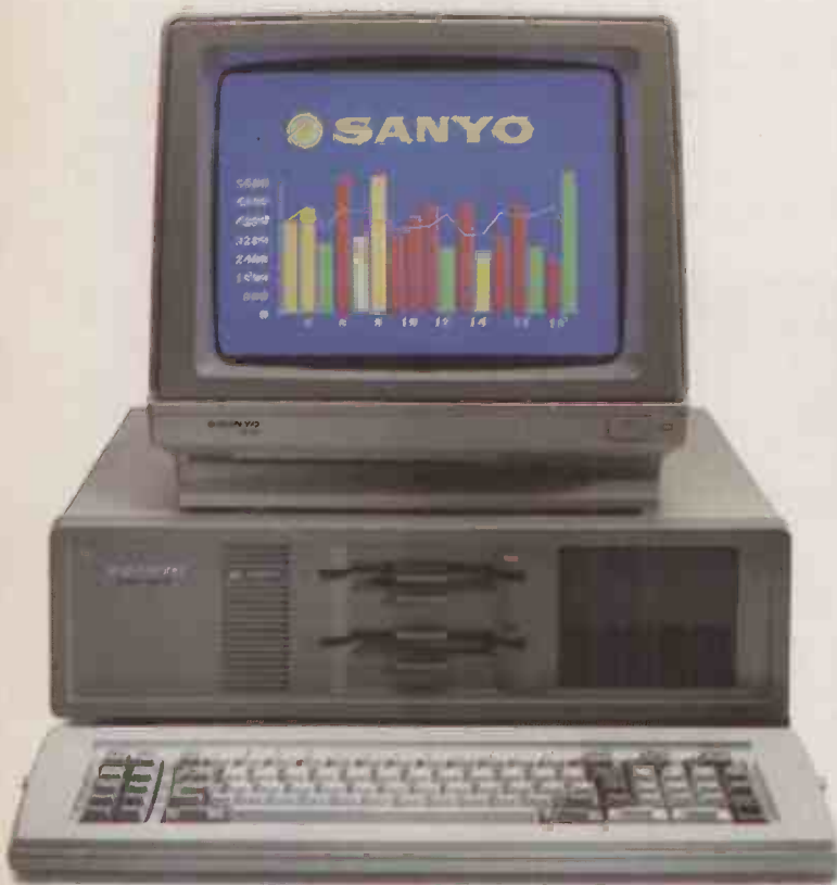
MBC 885 £1,390 + VAT.* MS-DOS 2.11. 256K RAM expandable to 640K. 2 x 360K drives. RGB colour/mono outputs. Centronics printer port. Seven IBM-compatible expansion slots. Provision for hard disk. Twice as fast as IBM PC. Free Wordstar 2000 software. Full IBM compatibility.
