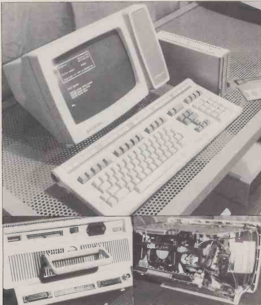
Top: Headstart has the same character definition set as the IBM PC's green screen. Above left: the expansion ports lie at the back of the screen/system box. Above right: the electronics are packed tight inside the VDU casing, leaving no room for expansion cards.
