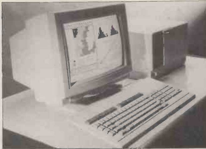
Bit-mapped graphics are handled by a dedicated 80186 chip.
