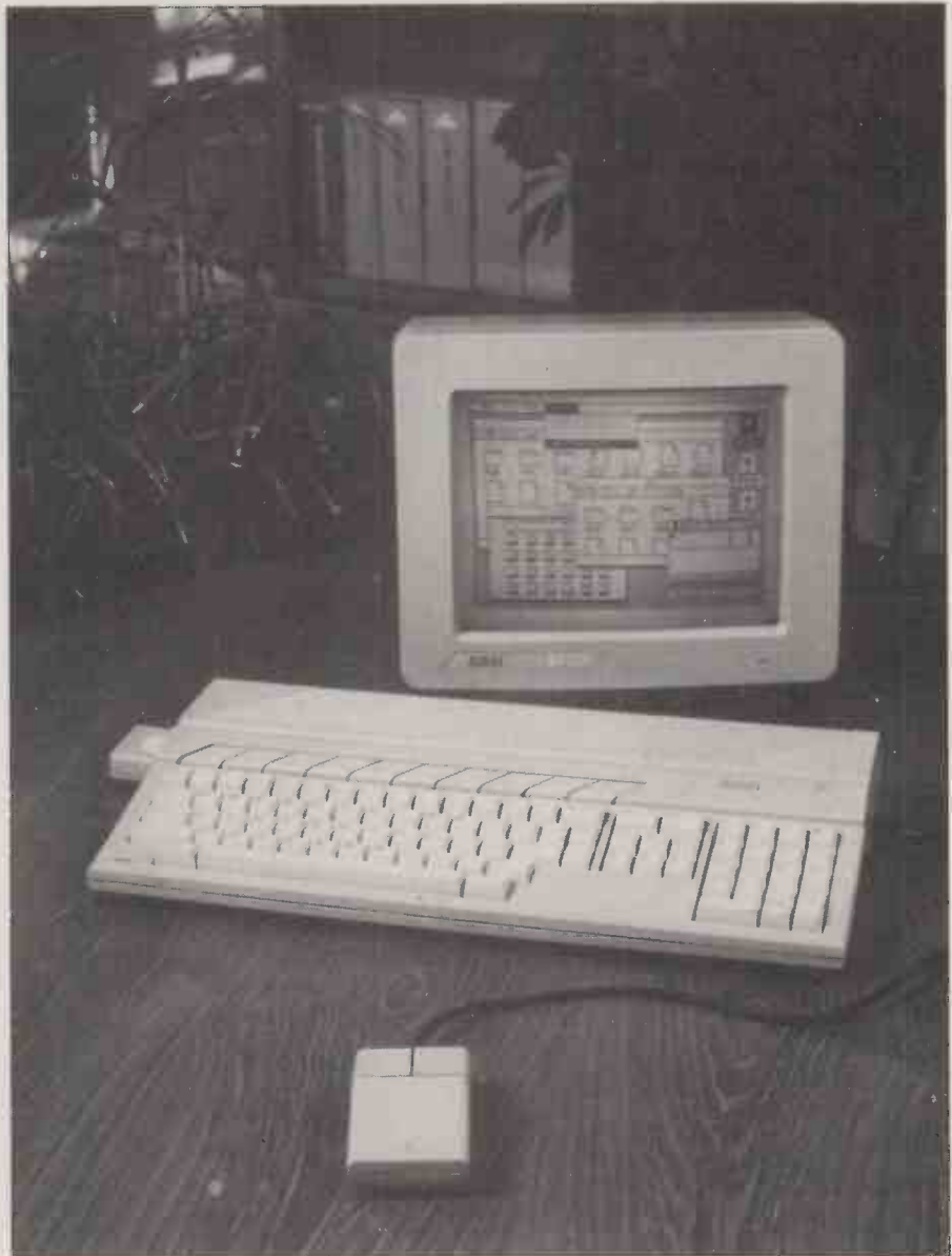
The 520ST provides a Mac-like user interface and a 68000 processor for under £700.
