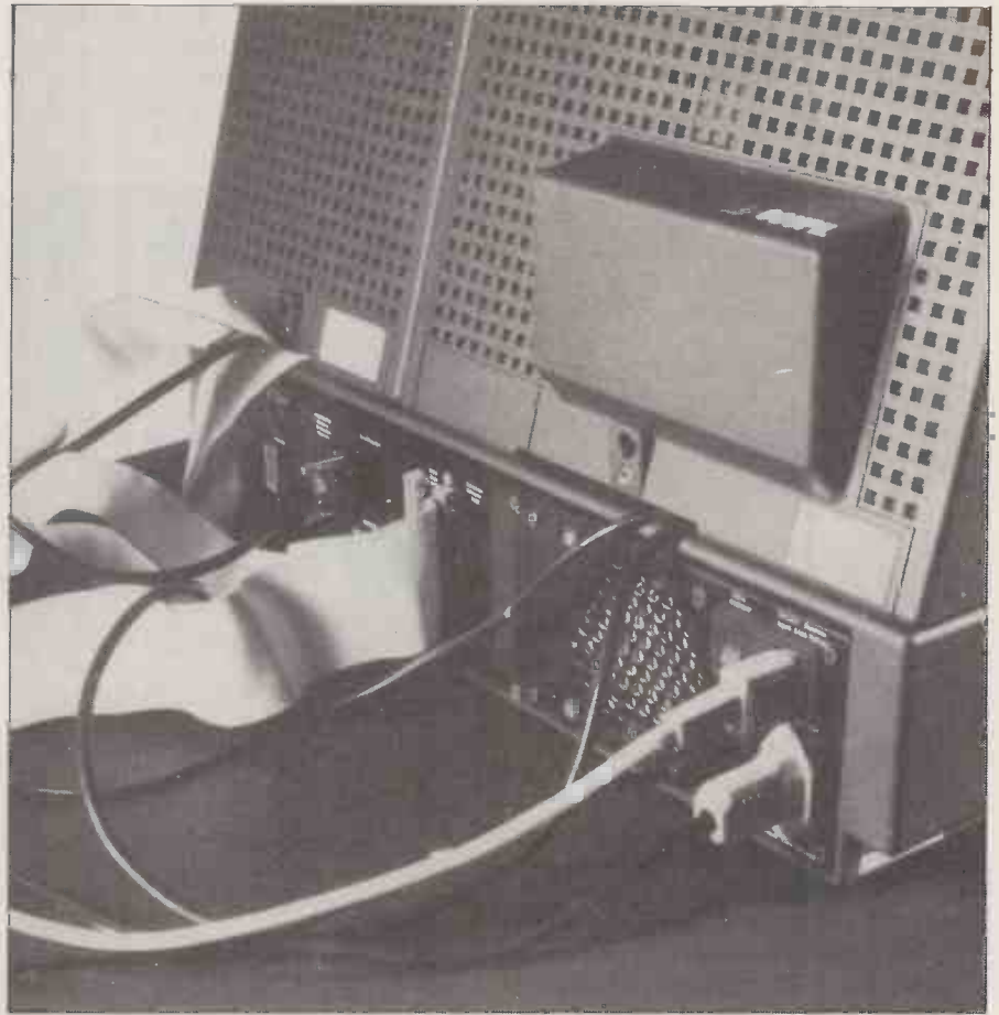
Centronics and RS-232 ports are sited at the back of the system box.
