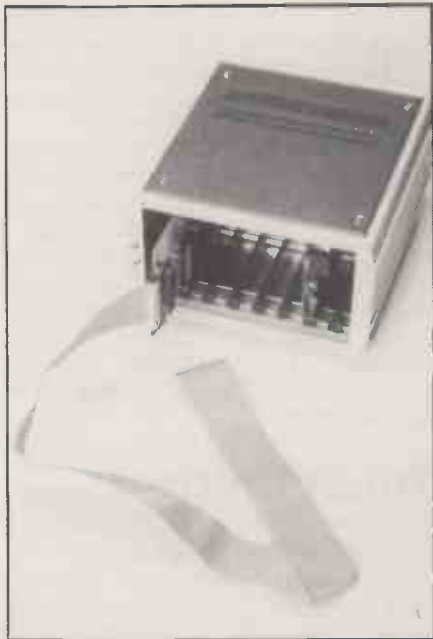
CMS mini-rack development system.
