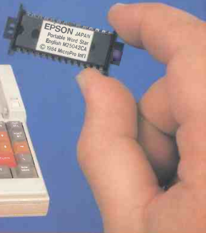
Below: The compact PX-8 runs CP/M software and offers WordStar on a ROM.
