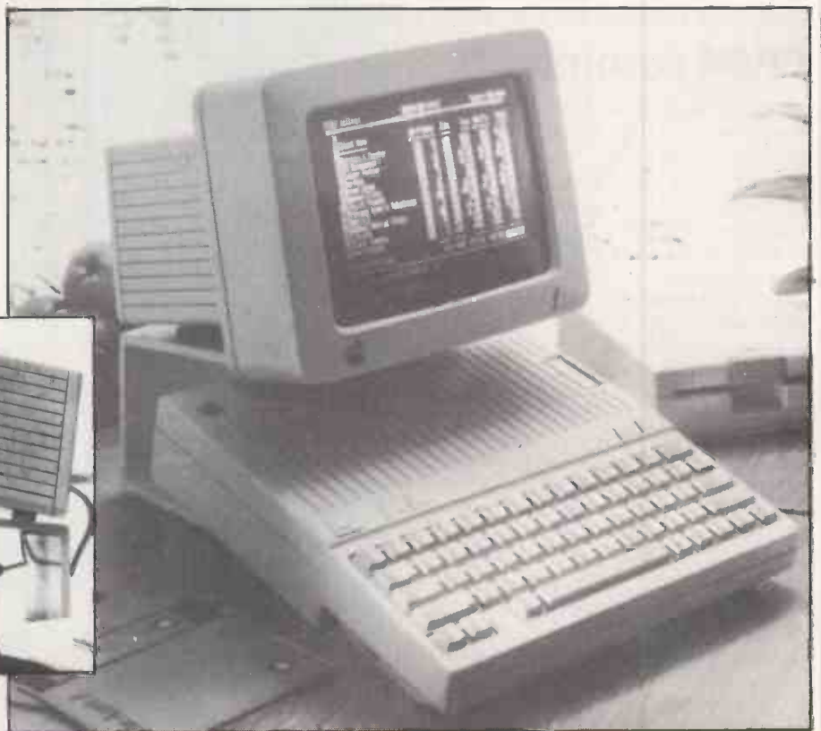
A half-height floppy drive is built into the side of the IIc. The monitor and mouse are optional.
