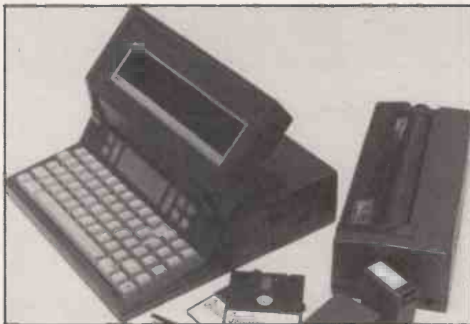
The Galivan portable micro has an add-on printer which uses a thermal ribbon and ordinary paper which combine to produce correspondence-quality results.
