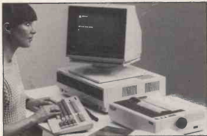
This is the Sharp MZ-3541. It has two Z-80A processors in it, so it isn't exactly going to set the world on fire. However it does offer the user access to a wide range of tried and tested software through its CP/M 2.2. It is available in monochrome at £1,795 and colour at £2,450. For details contact Sharp Electronics. Telephone: 061-205 2333.
