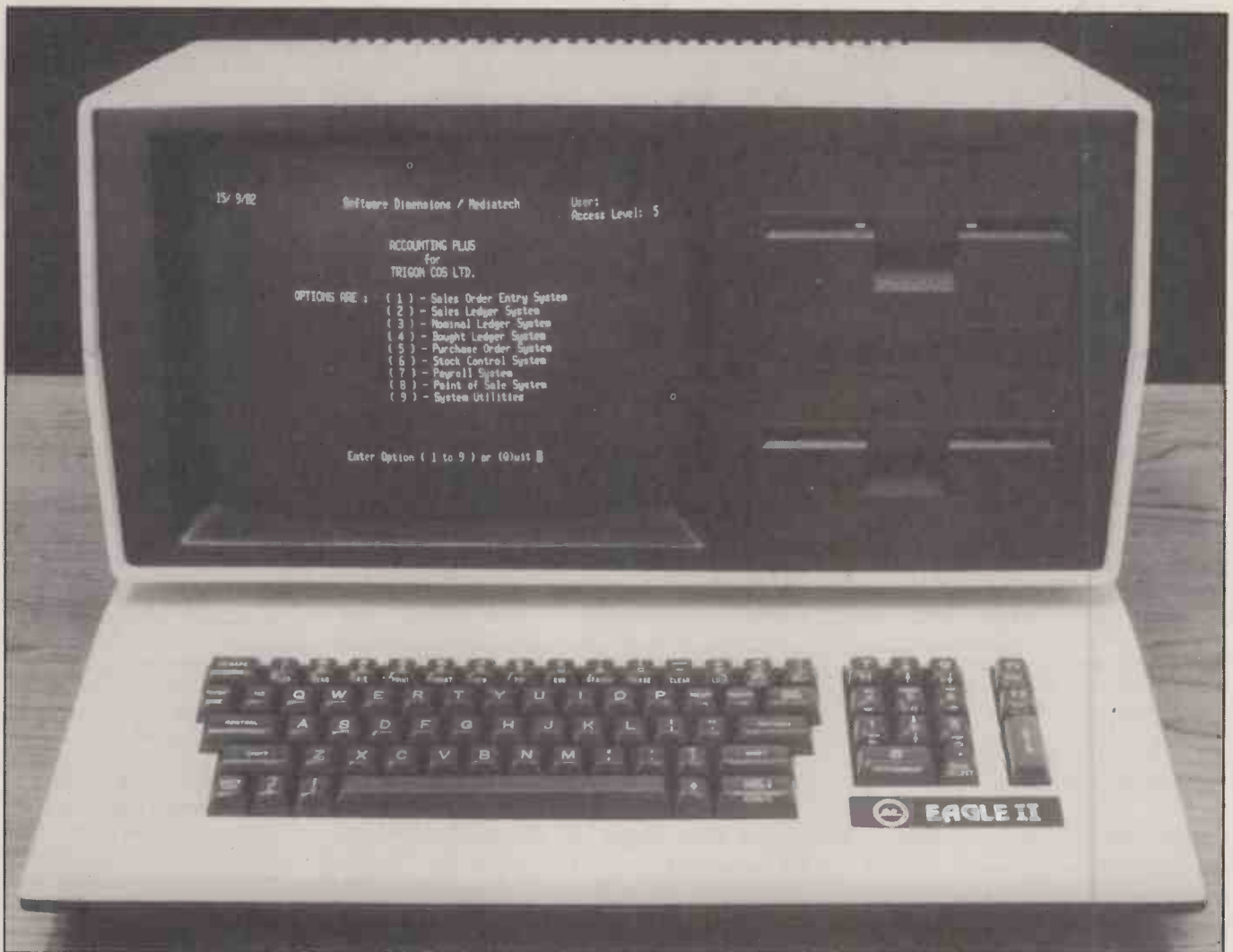
The non-detachable screen has a green phosphor and displays a lower-case character set.
