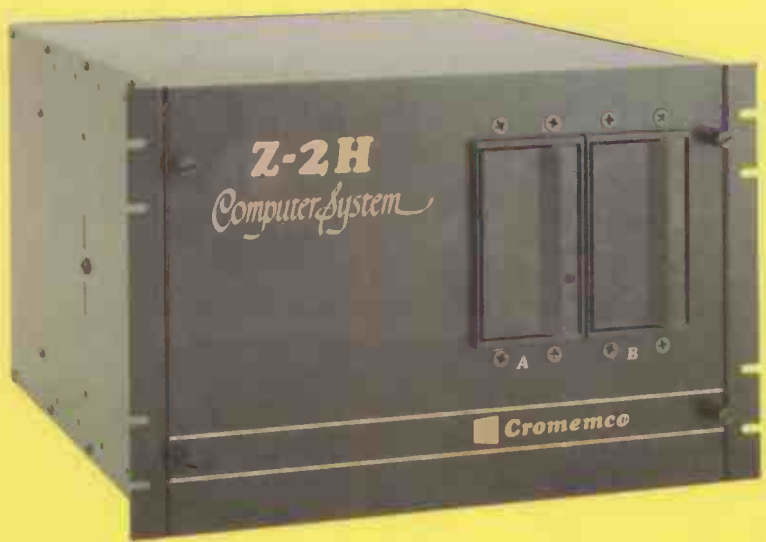
Cromemco Model Z-2H hard disc computer. 10 megabyte hard disc, 2 floppy discs, 7-80 computer and 64K memory. MicroCentre price £5,326.
