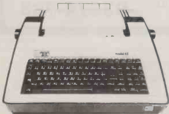
TELETYPE MODEL 43 10/30 C.P.S. Keyboard send/receive terminal.
