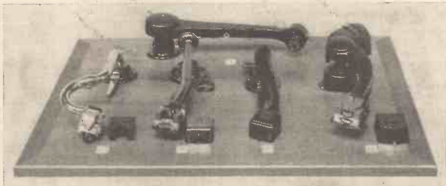
This is an exhibit prepared by H.M.V. for the Science Museum to illustrate the development of gramophone pick-ups. The instrument at the back is an oil-damped pick-up. Then, left to right, we see a magnetically-damped type; a pick-up with a counter-weighted arm; the standard pick-up fitted to H.M.V. radiograms with the exception of the Model 801, the pick-up for this being on the extreme right.
