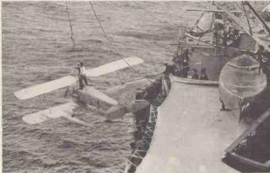
"Queen Bee" machines have so far been largely used for gun practice at sea. Here one is being hauled aboard H.M.S. "Neptune" after a successful flight.
