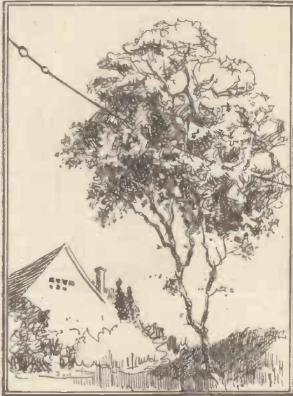
Don't erect your aerial in such a manner that the horizontal portion is brought into contact with the branches of trees.
