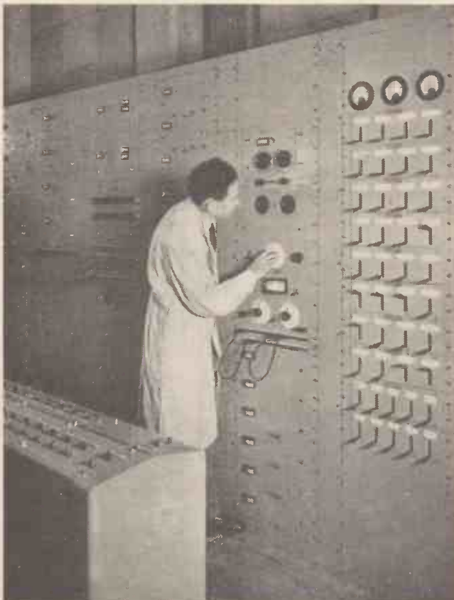
This photograph, taken in the control-room at the Alexandra Palace, shows the amplifiers used for the sound-tracks. On the right are the switches for the various amplifiers.
