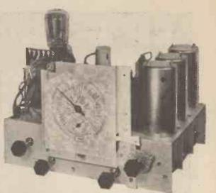
In this chassis view of the McMichael 362 all-waver the small "band-spread" pointer, which is so valuable on short waves and which works rather like the second hand of a watch, can be seen below the main pointer.
