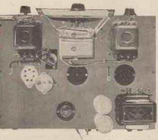
This view looking down on the top of the chassis shows the clean, straightforward layout. The rearmost valveholder is for the rectifier valve.
