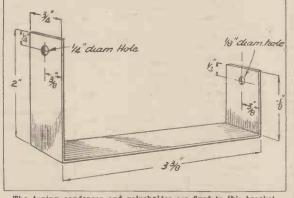
The tuning condenser and valveholder are fixed to this bracket, and these two components support the remaining parts, as will be clearly seen by reference to the wiring diagram.
