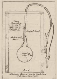
How the coupling loop is arranged on the inside of the container. The end marked "front" is that to which the panel is fixed.
