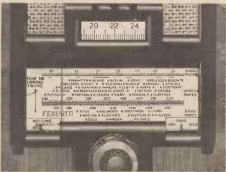
This close-up picture of the tuning arrangements of the Ferranti "Arcadia" receiver shows clearly the optical effect of the Magnascopic dial. The projected scale is, of course, the one above the main tuning scale,
