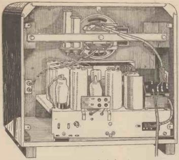
This is one of the first sets ever to be produced with which the sound side of the television programmes can be received in addition to short. medium and long waves. It is the H.M.V. Model 481.
