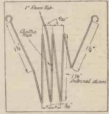
These are the dimensions for the coil, which is made with No. 18 gauge tinned copper wire. It should be borne in mind that the slightest variation from these dimensions may alter the wavelength coverage to a large extent.
