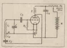
Fig. 2.—Reaction control by voltage variation on the anode avoids hand-capacity effects and prevents reaction affecting tuning.
