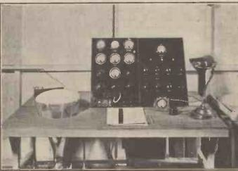
A close-up view of the Ediswan cathode-ray tube tester to which reference was made last week.
