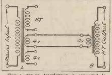
How a step-up transformer is connected to the L.T. winding of an ordinary mains transformer.
