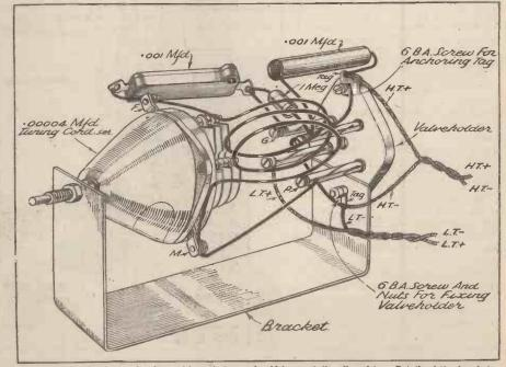
The wiring is simple, but the form of layout shown should be carefully adhered to. Details of the bracket will be found on page 415.
