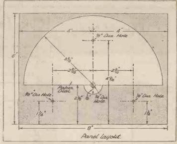
Here are the dimensions, you will need for drilling the panel and cutting the paper scale.
