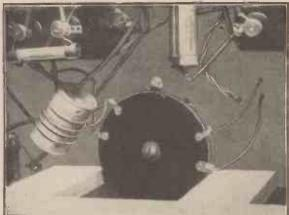
This close-up shows clearly the method of arranging the 7-metre coil and the wave-change switch.
