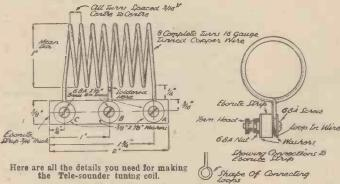
only eight turns, when the coil is released from the former the turns spring out to a slightly larger diameter. The excess over the eight turns is used for making the connecting loops at the ends of the coil.
