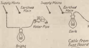
These two sketches are reproduced from W. S. Ibbetson's well illustrated book on "Accumulator Charging and Maintenance and Repair." The top one shows the method of finding the earthed main, and that on the right depicts an accumulator joined to the terminals of a lighting switch for charging purposes. The switch, of course, must be "off."
