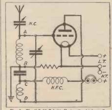
Fig. 3—The "Split-Colpitts " circuit which oscillates freely. It is a good short-wave circuit.
