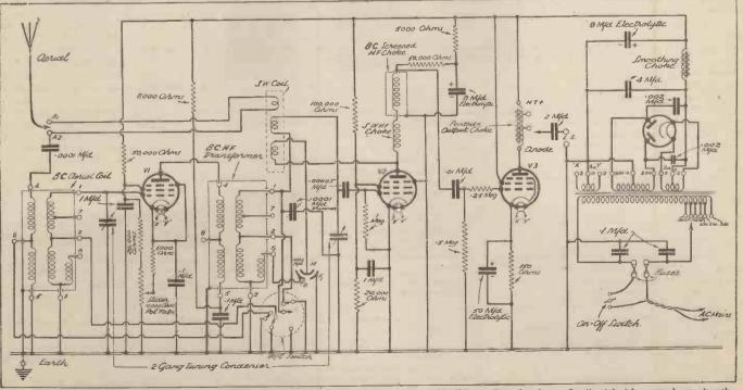
As can be seen the circuit employs three pentodes, these giving absolutely maximum sensitivity with this number of valves. On the television sound wavelength the set functions as a detector and L.F., a simple switching scheme providing an instantaneous change-over from one waveband to another.
