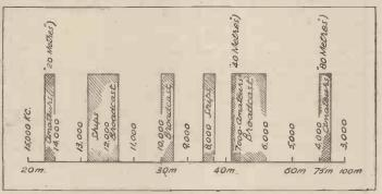
Fig. 2. Showing the allocation of the waves above 20 metres which will help you when tuning-in on the short-waves. Fig. 3 (right) has been drawn to guide you on the most suitable times to listen on the various wavelengths.
