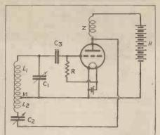
Fig. 1.—The figures 1, 2 and 3 show the evolution of the "Tele-sounder " circuit. First of all we have a normal reaction circuit.
