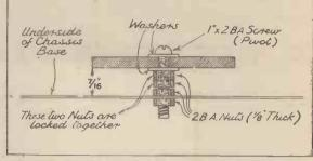
The switch disc moves on the threaded-rod spindle, which is secured by nuts to the metal chassis.
