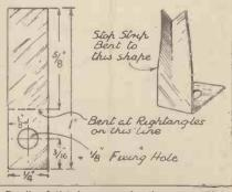
Details of the long-wave locating stop. The strip engages with a "V" cut in the wave-change switch disc. The
