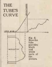
The effect will be rather like an under exposed print—greys and whites, but no contrast. On the other hand, if the bias is set too high an appreciable value of signal will be required to bring the curve up the bend, and the picture will suffer from . an excess of . black, giving heavy shadows.
