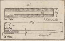
Fig. 2. Details for making the test prods. In-sulated prods of this type can also be bought ready-made.
