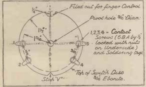
The ebonite disc, which is turned to change wave-ranges, is pre-pared in accordance with these dimensions.
