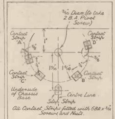
The above-baseboard wiring and layout. It should be noted that certain terminals on the coil units are not used. These are 6 and 7 on the aerial coil and 7 and 8 on the H.F. transformer. The sketch on the right gives the positions of the contact strips beneath the switch disc.
