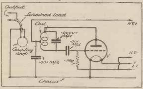
As in the case of the "Universal Oscillator" described in the November 28th Issue of "P.W." a "squegger" circuit is used. The coupling loop is attached to the oscillator case and is shown in position in the photo on page 415. The pitch or note of the oscillation can be varied by adjusting the H.T.
