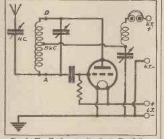
Fig. 4.—The Hartley circuit. As in Fig. 3 the tuning condenser is "live " on both sides, but this difficulty can be overcome by fitting an extension rod so as to set the condenser well back from the panel.
