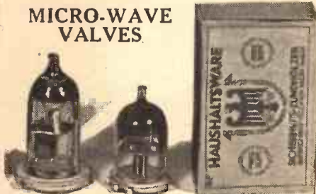
Two of the latest Telefunken valves for micro-wave work. The small size of the valves will be readily appreciated by comparison with the match-box.
