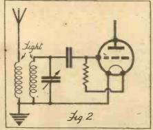
Fig. 1 shows direct coupling with a variable condenser. It is quite good so long as the capacity is kept low. An untuned aerial coil, as in Fig. 2, has many advantages, including quieter background and greater freedom from hand-capacity effects. The tuned aerial coil scheme of Fig. 3 provides a very good degree of selectivity.
