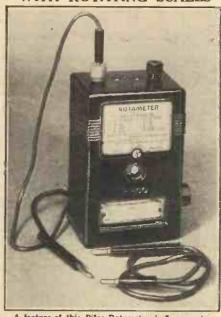
A feature of this Pifco Rotameter-de-Luxe meter is the provision of scales which automatically change with the operation of the range-change
