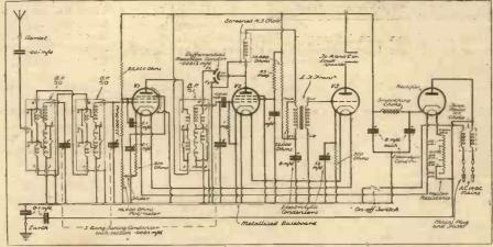
[Band-pass aerial tuning, H.F. transformer coupling and a specially arranged L.F. circuit combine to give high quality and excellent selectivity in this latest any-mains three.
