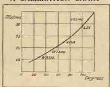
A wavemeter calibration chart is easily obtained by logging a few known stations, and provides a means of identifying unknown transmissions.
