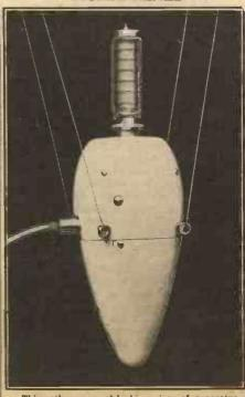
This rather unusual-looking piece of apparatus is an Edison Bell microphone with a B.B.C. streamlined amplifier.
