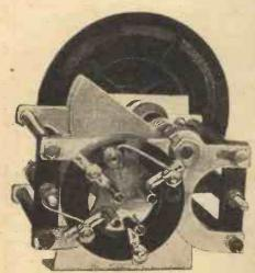
Here is a view of the absorption wavemeter described on this page. The coil is inserted in the valveholder bolted on to the tuning condenser. These two components are the only ones required, apart from three plug-in coils.
