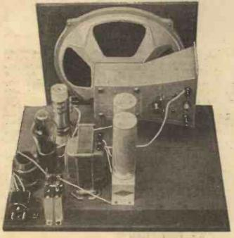
allows the sensitivity to be increased where a particularly distant station is required. Since the first valve is a multi-mu pentode it can be controlled by the bias potentiometer to give pre-detector volume control-an
