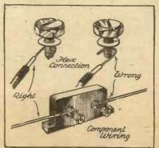
Whether wires fit under screw heads or ordinary terminals, there is a right and a wrong way of twisting them round the shank so that the wire will not be squeezed out in the tightening up process.
