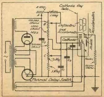
The exciter circuit used for producing the necessary voltages for the cathoderay tube. Note that the positive is earthed, not the negative side, as is usual in radio circuits.
