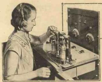
Coil-testing in progress in the Cossor factory. Every coil is tested many times, to ensure correct electrical characteristics and for mechanical soundness.
