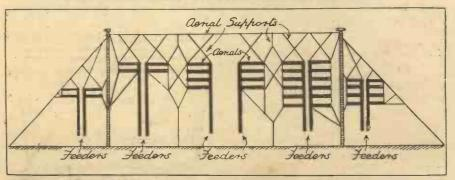
The short-wave aerial systems at Daventry have been completely transformed. All the original "beam" aerials, with their reflectors, have been scrapped, and horizontal di-pole aerials as shown in the above diagram have been substituted.
