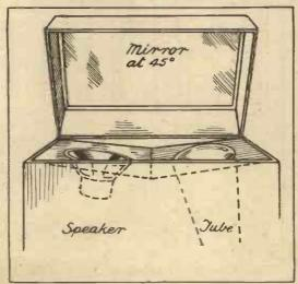
The idea behind this arrangement is to make the sound appear to come from the same point as the picture by reflecting both sound and vision from the mirror.
