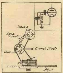
Keep the connections between coil, condenser and valve as short and straight as possible.
