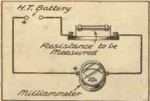
Using a battery and milliammeter to test a resistance. Start with a low voltage and gradually increase till a suitable reading is obtained.
