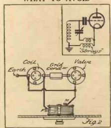
Indirect wiring, such as shown here, may easily be the cause of bad hand-capacity effects.
