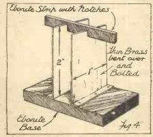
An ingenious aerial-coupling condenser designed by a reader for short waves.
