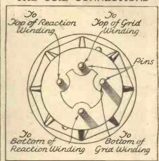
This diagram shows how the windings of the four-pin coils are joined to the pins on the base of the former. Full details of the windings were given in the June 8th issue of "P.W."
