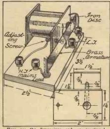
Here are the dimensions and construction features of the mains unit switching device. I magnet is wound with 18 gauge D.C.C. wire. constructional
