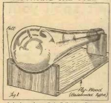
A simple wooden cradle is all that is really necessary to accommodate the cathode-ray tube in safety.
