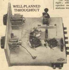
The detector valve holder (VI) and the "neutralising" type condenser are mounted on small blocks of wood to keep them about a quarter of an inch above the metal-coated baseboard.
