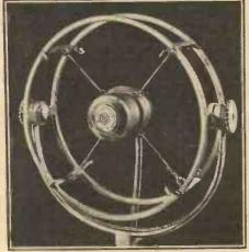
One of the microphones used by the B.B.C.—the E.M.I. moving coil type. Note that it is suspended on a swivel stand so that adjustments can be made to its position.
