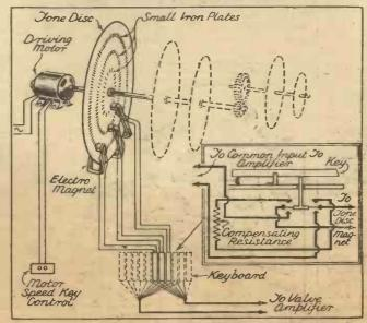
The various notes are developed by means of rotating discs having iron plates on them which pass through the poles of electro-magnets. The inset diagram shows how the operation of the playing keys cuts out compensating resistances when the "pick-up" outputs are switched over to the amplifer.
