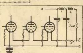
Fig. 1a, above, shows the connections required when the heater voltagedropping resistance is in the positive mains lead, while Fig. 1b, to the right, shows this resistance in the negative lead.
