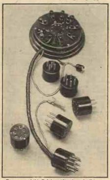
By means of this Bulgin outfit valves of all types may be tested. Each connection is split so that a meter may be inserted.
