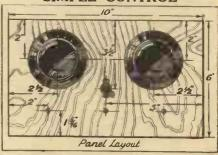
Simplicity is the keynote of the design. There are only two real controls, viz., the tuning dial on the left and the reaction dial on the right.
