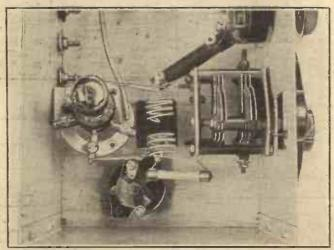
This photograph shows the tuned circuit of a 5-metre receiver. Although this uses a different circuit from that shown on the preceding page, the same principles in wiring have been observed with regard to the coils.
