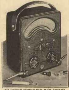
Universal AvoMeter made by the Automatic Winder and Electrical Equipment Co., Ltd. It has 36 different ranges in all.
