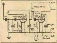
The circuit is a straightforward two-valve arrangement consisting of a triode detector followed by a resistance-coupled L.F. stage.
