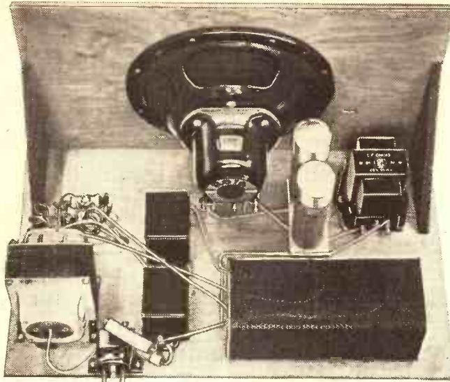
The power pack and the speaker baffle fit into the top portion of the receiver. The hole through which wires pass to the main portion below is partly hidden by the leads running to the rear of the power transformer.
