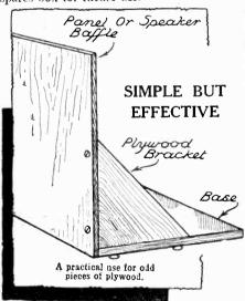
In fact, one useful method of utilising such odd pieces of wood is in the form of panel brackets for fixing either a panel and baseboard or baffle and base, as shown in the diagram.
