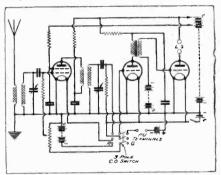
The 3-pole change-over switch shown in this diagram is wired up so that when it is in the central (or "off") position or when over to "radiogram" it automatically disconnects the S.G. valve's grid-bias battery and filament supply
