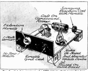
Fig. 2.—"A fair specimen of a 1924 vintage short-waver," is how W. L. S. describes this receiver with its old-fashioned de-based valve.
