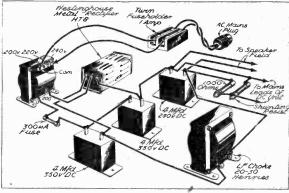
sufficient to prevent any trace of hum. If this should not be the case the 1,000-olms resistance in the converter provides a small degree of smoothing.
