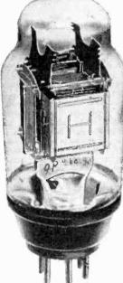
which allows the camera to "see through" the gettering of the valve) of the new Hivac QP.240. Note the intricate electrode assembly, and the sturdy construction. ment connected to No.
