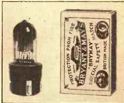
This is one of the new midget valves which are available in the Marconi and Osram ranges. It will be seen that the base is of the pinless type.
