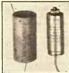
The two types of Dubilier condenser described this week, and recommended to constructors, after tests by our Technical Editor. The construction is shown in this photograph.
