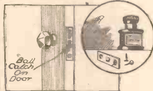
Marking the exact position of a hole to take a ball catch.
