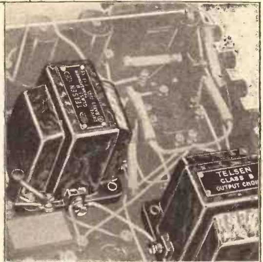
The illustration above shows the position occupied by the Telsens 'Class B' Driver Transformer and Output Choke in the built-up P.W. 'S.T.500.'
