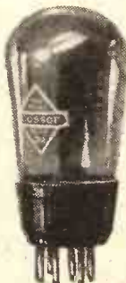
The Class B valve is unlike the other battery types in that it has seven pins. This is because it is really two valves in one bulb.
