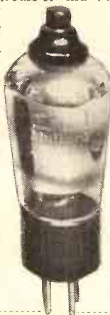
The screen-grid valve has a terminal on the bulb as well as four pins in the battery type, or five pins in the mains version.
