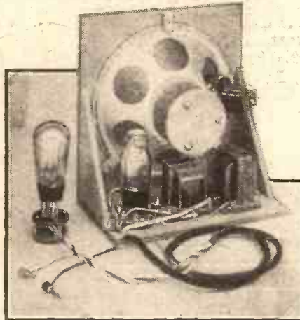
The adaptor which connects the speaker unit to the set is seen to the left of this photograph. The output valve is placed in it, as shown, when the unit is in use.
