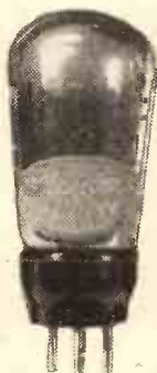
This is an ordinary battery three-electrode valve suitable for use with a 2-volt accumulator. Valves of this type are employed as detectors and low-frequency amplifiers.
