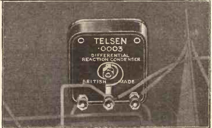
Illustration below shows the position occupied by the new Telsen Differential Condenser in the built-up S.T.500.
