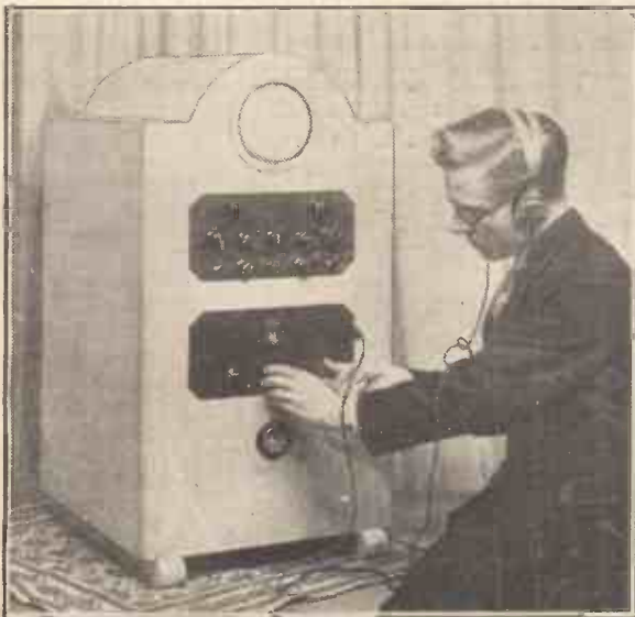
Tuning the "vision" receiver in the complete Cathode-Ray Television outfit. The special cabinet shown will be described next week.
