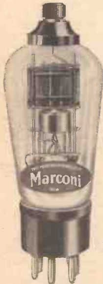
Fig. 1.—This valve is developed especially for automatic volume control, and consists of one triode and two diode valves in one bulb.
