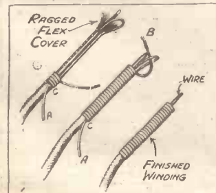
Greased fishing line, finished with shellac, forms the basis for this neat finish to untidy flex leads.
