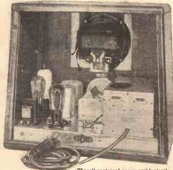
The self-contained power unit is clearly shown to the right of the photograph, which also shows the compact and clear-cut layout.
