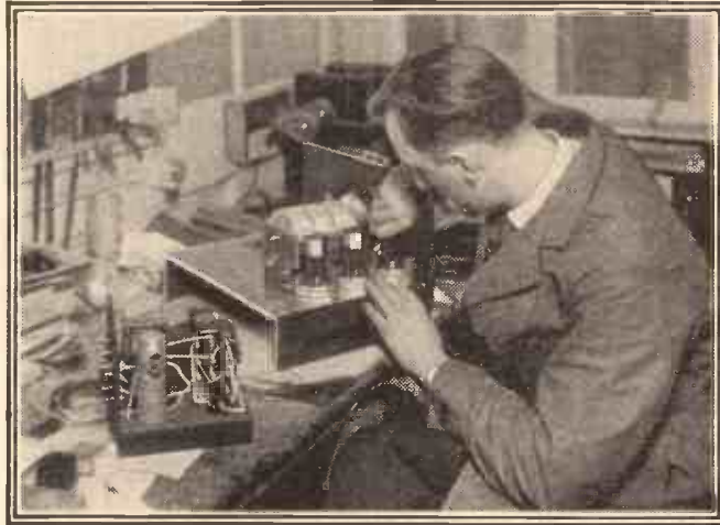
This further view of the "Double D.T." receiver shows the H.F. end with the three matched coils in the process of being wired.
