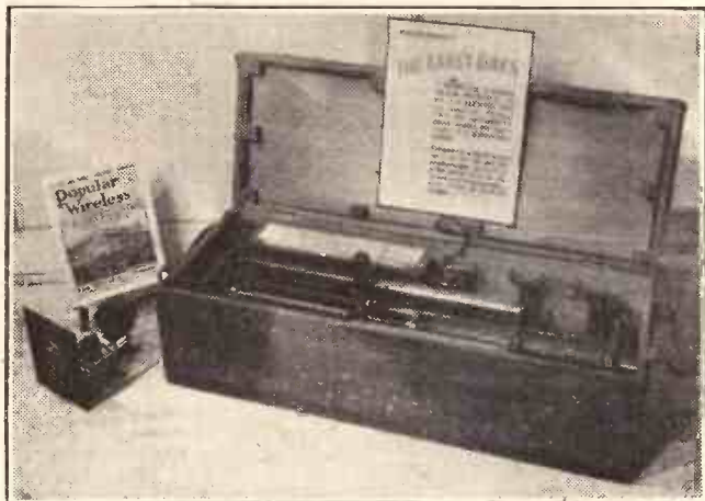
One of our exhibits which caused much interest at Olympia. A Fleming wavemeter, used in the earliest days of wireless, and the corresponding apparatus which is used to-day.
