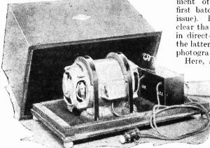
The Wates Rotary Converter made by The Standard Battery Co.
