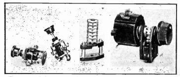
The on-off and change-over push-pull switches, a plug-in R.D. resistance and the combined volume control and on-off switch.
