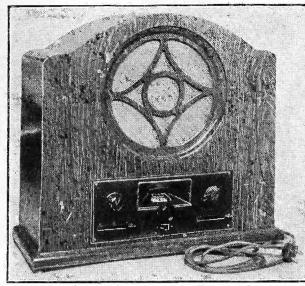
An inductor type loudspeaker is incorporated.
