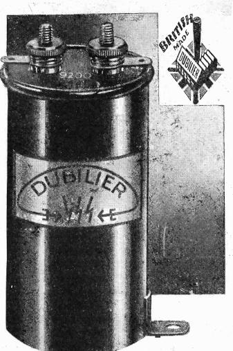
This is the Type 9200 condensor intended primarily for use where lowest radio frequency impedance is required. Ideal for by-pass purposes in H.F. circuits. Working voltage 250 D.C., tested 500 volts D.C.- Capacities from .01 mf. to 2mf. Prices from
