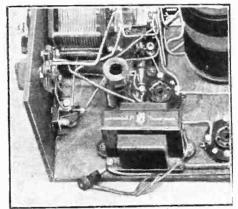
When wiring the volume control in a circuit such as this, take care to keep the leads from the components concerned as short as possible. That is, if you want pleasing results 1
