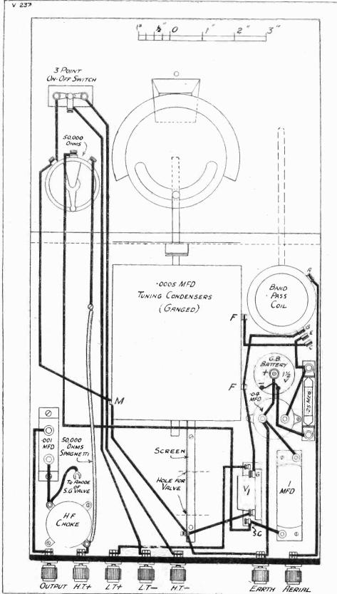
The wiring is particularly simple, there being a mere handful of connections. When joining up the "Square-Peak" coil you will find the lettering for the various terminals on the metal hand round its middle, and not near the terminals, as you might at first expect.
