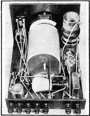
The two-gang condenser is totally enclosed in the metal can seen here, and besides effectively screening this vital component, it assists here, and besides effectively screening this vital component, it assists considerably in separating the anode circuit of the S.G. valve from the rest of the unit.
