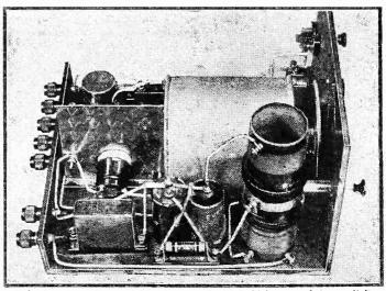
This view shows the special hand-pass coil with built-in wave-change switch. The windings of this coil are balanced up in such a way that with a 04-mfd. coupling condenser 9-kc. separation is obtained.
