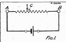
If a resistance is connected across a battery as illustrated above, any desired voltage, up to the maximum of the battery, can be tapped off with the slider. Hence its name—a potential divider.
