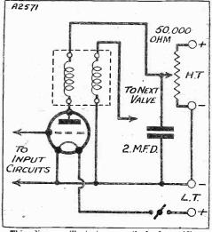
This diagram illustrates a method of providing (he 1st detector of a super-het. with a variable H.T. tapping.
