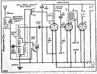
The Moderator coil and condenser bring the aerial circuit into resonance at "medium-wave" frequencies, and thus enable the maximum of power to be developed.
