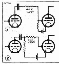
The top diagram shows the wrong way to connect a grid stopper in an R.C.C. circuit, while the ... bottom one illustrates the correct method.
