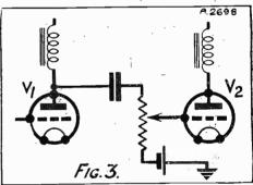
When a potential divider is used in this manner as an L.F. volume control there will be no voltage variation due to load. This is because for all practical purposes there is no current flowing in the grid circuit.
