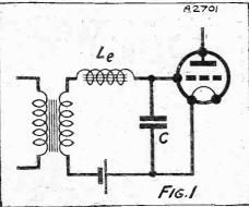
What is known as the magnelic leakage of a transformer can be considered as an inductance in series with the secondary winding. Unless properly used, this inductance can completely spoil the response curve of a transformer.
