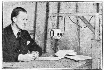
The great advantage of the condenser microphone is that the background noise is much less noticeable than with the Reizz type. The instrument shown in the above photograph is of the latter pattern.
