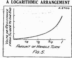
The advantage of a volume control wound on the logarithmic principle is that the variation in volume is proportional to the amount the knob is turned.
