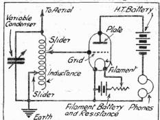
This ten-year-old one-valver had the tele-phones connected to H.T. negative, and used no grid-condonser or leak ! A modern one-valver would knock spots off it !
