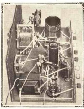
**COMPLETE STABILITY** High quality of reproduction at great volume is made possible by a combination of transformer and resistance-capacity L.F. stages and effective detector de-coupling.
