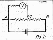
If current is taken from a potential divider, the voltage across that section of the resistance which is in use will drop considerably. (This explains why misleading race obtained when cheap low-resistance voltmeters are used, for testing mains units employing such an arrangement.) decibel, or more shortly still a d.b. Decibels are really the logarithm of the ratio of powers, but we won't worry you more than to say the following.
