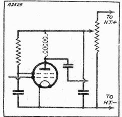
The potentiometer is arranged to control the anode voltage as well as that applied to the screen. This scheme has several advantages over the usual method where the screen voltage only is varied.
