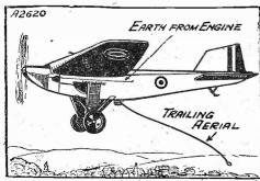
The engine and metal parts of an aeroplane constitute its radio "earth."
