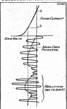
With the aid of this diagram Capt. Eckersley explains o J.M. why the anode current of a grid detector falls when a station is tuned in.
