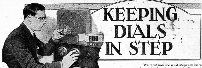
T will often be found that with receivers having two dials for tuning, the two dials do not keep in step over the whole of the scale, but fall out at the top and the bottom. This makes tuning more difficult for the inexperienced. Before seeing how this can be avoided, we must see exactly what happens.
