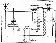
The Phonotrap is highly efficient both as a wavetrap and a crystal receiver.
