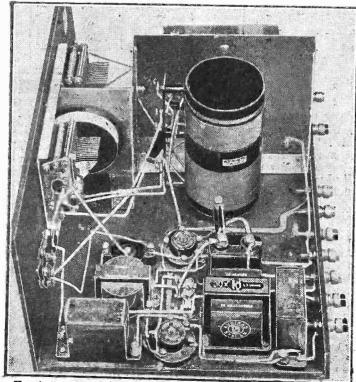
Here is the compact L.F. end. On the right of the second valve is the output choke and condenser, and to the left of it the L.F. transformer and a by-pass condenser.
