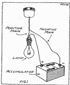
By connecting the accumulator in this manner you illuminate the room while you charge the battery! With an H.T. accumulator, however, there would be a big voltage drop and the lamp would glow but dimly.
