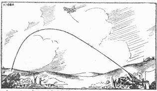
an extremely useful job for radio-equipped aeroplanes is to spot? for the big guns. The observer in the machine wirelesses the gunners and tells them if their shells are hitting the mark, and gives them information that will assist in finding the range.
