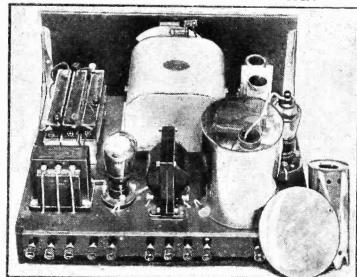
A feature of this Ferranti receiver is its simple but completely effective screening.
