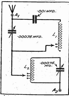
Last week we gave only the "components" for a Brookmans Rejector, and above these are shown "wired up" into a complete circuit. DID YOU GET THE WIRING RIGHT?
