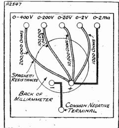
Here you see a back view of the panel, showing how the various resistances are connected. When building this instrument it should be remembered that its accuracy depends on the accuracy of the spaghetti resistances.
