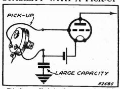
This diagram illustrates the answer given last week to J.M.D. (Belfast), explaining how a pickup may be earthed through a condenser to improve stability.
