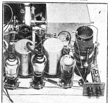
In spite of the receiver's advanced nature, i. s not a all a difficult matter to carry out the preliminary adjustments. Once these are effected the tuning-in of distant stations is as simple as receiving the local on a crystal set.
