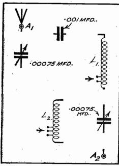
This week we have an unusual "missing link"—all the parts are shown, and the test is whether you can fill in the missing "wiring" to join up a Brookmans Rejector.
