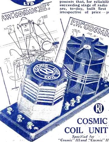
This component combines in one complete unit, coils for long, medium and short waves, ensuring easiest fixing and most compact set assembly. A fact of paramount importance is the skeleton construction of the short-wave coil former, which reduces dielectric losses to a minimum—a vital point in these circuits. Every individual coil is carefully tested, before release, on the "Cosmic" III circuit, and
