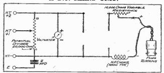
This is a simple unit for deriving H.T. from D.C. mains, but three of the "components" have been omitted. Can you fill them in correctly? LOOK OUT FOR THE ANSWERING DIAGRAM NEXT WEEK.
