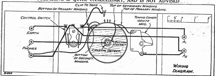
Providing you clean the lead ends thoroughly and screw them down moderately tightly the contacts so formed should never give the slightest trouble—and that cannot be said about even expertly-made soldered joints,
