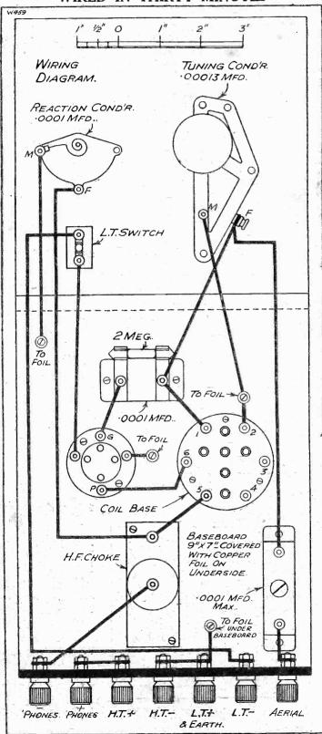
The wiring of The "W.L.S." Short-Wave One offers no difficulties even to the novice. The whole job, right from start to finish, need not occupy more than half-an-hour at the very outside. Follow this diagram carefully, and you will be sure of success.
