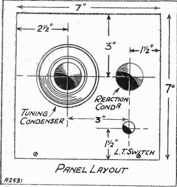
The panel is quite a small affair, and there are only three controls. Most panel components are arranged nowadays for one-hole fixing, so it should only be necessary to drill the ebonite at the places marked. All the measurements are clearly indicated.
