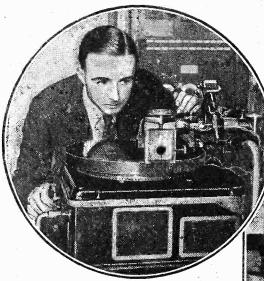
In the above photograph we see the H.M.V. recording engineer setting the cutter on the wax blank before switching on the red light to signal the commencement of the actual recording. This process follows the one illustrated on the extreme right—the polishing of the wax blank prior to recording on it. A very high polish is essential.
