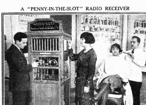
This automatic slot machine for radio programmes is being tried out in a barber's shop in Philadelphia. It is a five-valver which will work from mains or batteries, and a red light comes on as a warning about a minute before it stops, so that one can insert another coin in time to avoid missing a desirable part of some item. It should be a bit better than the usual papers that are provided to while away the time until one's turn comes to respond to "Next, please !"
