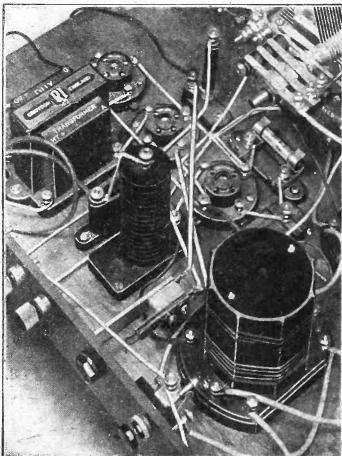
Tuis is a close-up of the pick-up jack inserted in the original model of the "Cosmic" Three. The jack is an ordinary break type, such as the Igranic P.62, known as a "single circuit closed" jack.
