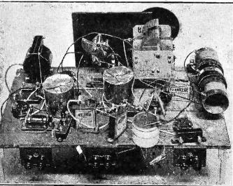
This is NOT the way a constructor should hash up one of our circuits ! However, this photo is of historic interest, for it shows one of the earliest experimental models of that very successful "P.W." set "S.Q. 22 Star. Note the "home-made ?? coil screens.
