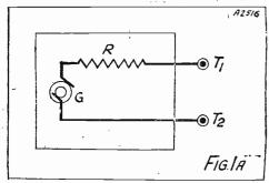
Our Chief Radio Consultant explains to a Leéds reader that the valve should be considered as the equivalent of the factors inside the square—a generator of variable frequency in series with a resistance.
