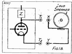
Here is a typical output circuit, as referred to in the reply to the first question. If a pentode is used instead of a 3-electrode valve the voltage drop across  $T_1$ ,  $T_2$  is accentuated as explained.
