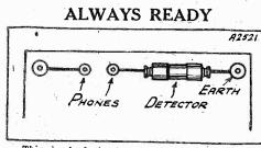
This simple device transforms a valve set into a crystal receiver.
