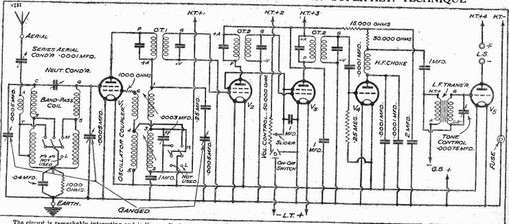
The circuit is remarkably interesting and is the result of many weeks of intensive research. The first valve is of the double-grid type, and works as a combined oscillator and first detector, with a band-pass feed from the aerial. Two intermediate S.G. stages are employed, and the second detector, which is an ordinary triode, is followed by a single stage of power amplification.
