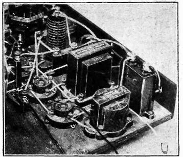
The L.F. choke and large fixed condenser in the foreground of this photograph of the low-frequency end of the original "Cosmic" Three, are the only com-ponents necessary to incorporate an output filter.
