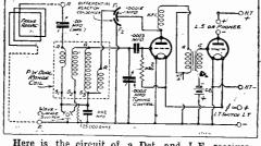
Here is the circuit of a Det. and L.F. receiver with two components purposely omitted. Can you fill them in correctly ? LOOK OUT FOR THE ANSWERING DIAGRAM NEXT WEEK.
