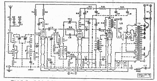
This is the theoretical circuit of the model 435. Note how the ganged volume control operates on both the S.G. and the pick-up circuits. Shunt-fed transformer coupling between the detector and the pentode ensures good L.F. response.
