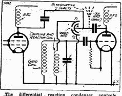
The differential reaction condenser controls volume as well as feed-back.
