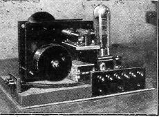
Many stations, use distinctive interval-fillers, on the lines of the B.B.C.'s '' doomp, doomp, '' and this is the apparatas used at Budapest, on 550 metres.
