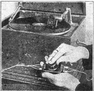
This picture shows the convenience of the H.M.V. pick-up head (Model 11) which can be fitted on to the existing tone-arm of a gramophone, and also the H.M.V. volume control previously mentioned. An alternative to the provision of a pick-up and gramophone motor, etc., is the use of the playing desk shown in the heading—one of the complete outfits made by the Gramophone Co.
