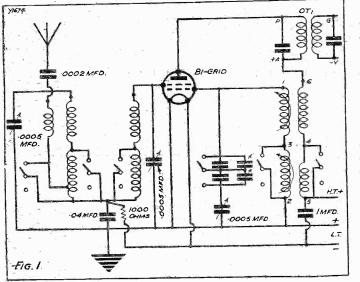
The initial tests were carried out with a bi-grid valve and tuned-grid windings, as above.
