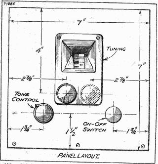
Although it is quite a large set, it only possesses a small operating panel. The tuning "peep-hole" and main control occupy the centre position, with the tone control and on-off switch just below, and on either side.
