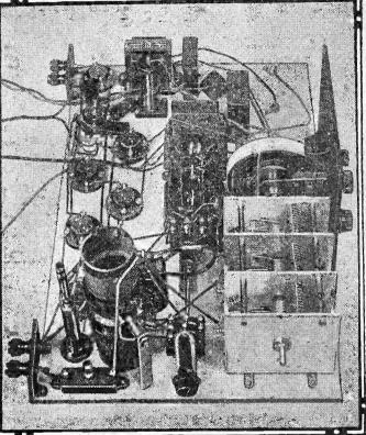
Here is the aerial end of the set, with the band-pass coil in the foreground. This time the ganged condenser is shown with the screening box cover removed, so that readers may see for themselves how the three separate sections are coupled up together.
