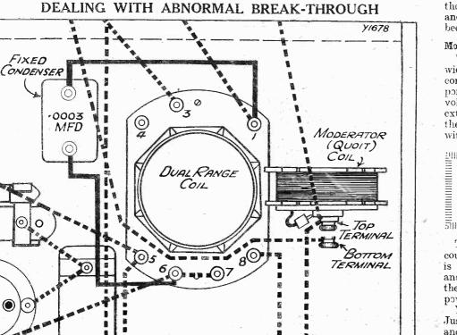
By inserting a small fixed condenser as shown it is possible to eliminate the last traces of "break-through " even in abnormally bad
