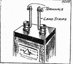
Besides making the accumulator more pleasant to handle, these terminal extensions tend to protect the leads from corrosion.
