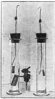
This fascinating experiment, which is explained in the accompanying article, demonstrates how radium will effectively neutralise the charge on a gold leaf electroscope.
