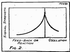
In the Armstrong circuit the area of instability which in an ordinary set is encountered near the point of oscillation, is wiped out altogether. The result is that reaction can be increased to a much greater extent and "the last ounce "of amplification extracted from the receiver. (The point marked X in the diagram is where oscillation commences.)
