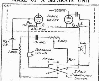
Here are the simple connections. All the components outside the dotted line can be incorporated in a special unit external to the set. The scheme is suitable for recording radio items as well as for record-making via a "mike."
