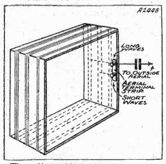
When making provision for connecting an outside aerial, it may be necessary to provide separate terminals for long and short waves; also, a series condenser is desirable.
