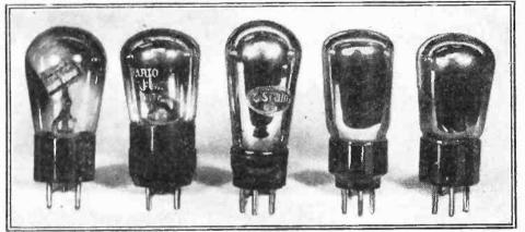
Some of the valves tried in the original "Cosmic" Three, and recommended as suitable for use in that set.
