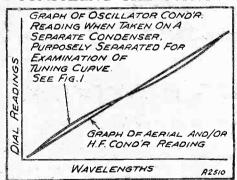
The curves of this diagram show the slight differences between a tuning condenser and the oscillator condenser of one single-knob super-het, in which the oscillator and tuning condenser are in step at the top and bottom readings.
