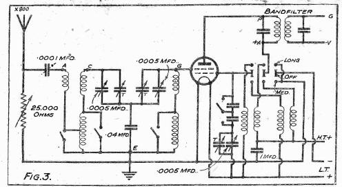
To obtain a balance on both long and medium waves two entirely separate fixed condensers are required in the oscillator circuit. Both condensers are connected in series and a switch arranged to short-circuit one or the other at will.
