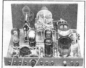
Here the valves and all coils are shown in position, and it will be seen that the latter are few in number and amazingly compact considering the wide wave range which is covered by the "Cosmic" circuit.
