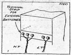
Showing how a terminal strip can be fixed to the outside of the receiver carrying the extra battery terminals.
