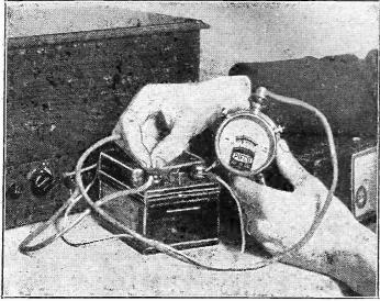
One of those handy little three-in-one meters such as the Pifco or Wates will prove invaluable for keeping your batteries up to scratch. Always test the L.T. and H.T. with the set switched on.
