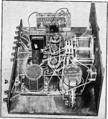
By merely pulling out that little switch on the terminal strip at the back, the set becomes at once a short-wave receiver instead of a two-band receiver of medium- and long-wave broadcasting. There is no coil-changing and only that one simple "transformation" switch!
