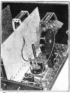
The use of modern valves in old sets of the neutralised type is not too straightforward, and may mean difficulty in obtaining stability.
