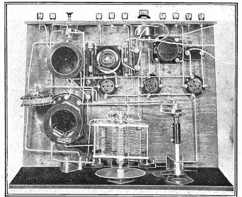
Extenser tuning, slow-motion reaction, divided capacity for simplined short-wave reception and single-dial tuning render the "Cosmic" Star easy and flexible in operation.
