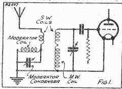
There is a loose inductive coupling through the short-wave coils, and the moderator condenser serves to tune the aerial circuit so that maximum efficiency at any particular wave-length is possible, as opposed to the losses usually associated with "aperiodic" aerial circuits.
