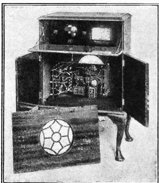
It is quite likely that new valves, particularly the output type, will need more high-tension current, and so you must always see that the mains unit in use is capable of supplying the needs. A good, big unit, as shown in this set, is desirable, so that there will be power in hand.
