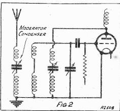
The aerial coupling provided by the short-wave coils is augmented for the long waves, and at the same time, and also quite automatically, the moderator condenser adopts a series position for regulating selectivity.
