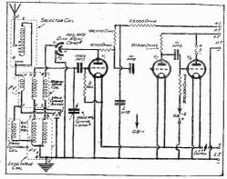
Here are the connections for a well-decoupled three-valver, but two "components" have purposely been omitted. Can you fill them in?
