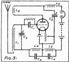
The modified short-wave Armstrong circuit used in the portable set described in this article. In many respects it resembles an ordinary regenerative single valver, but the main difference is the inclusion of the pair of quenching coils L4, L5, and condensers C3, C4, upon which the receiver depends for its extreme sensitiveness.
