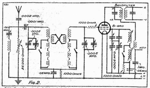
Originally used in a popular American single-dial super, this circuit is capable of very accurate ganging for medium-band working. Although there is bound to be a slight error, it is not sufficient to affect the sensitivity of the set, especially when employing band-pass tuning in the aerial circuit.
