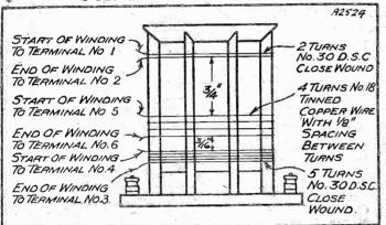
If you want to make your own short-wave coil, you will be able to obtain all the necessary details from this diagram. The ribbed former should be  $2\frac{a}{b}$  inches to the outside of the ribs.
