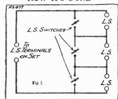
Three sets of loudspeaker terminals are provided, with a shorting switch across each pair. All three are connected in series, so by opening one or more of the switches the individual speakers can be brought into action at will.
