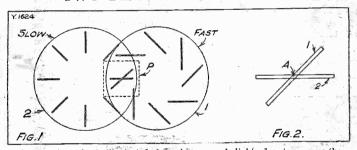
The scanning scheme illustrated above has several slight advantages over the single disc arrangement. But although the discs rotate at a much slower speed, it still has the disadvantage that it is "mechanical."
