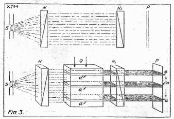
The method of scanning shown in diagrammatic form here, is fully explained in the accompanying article. It is claimed to be a tremendous improvement over all mechanical methods, and makes use of a piezo-electric crystal.
