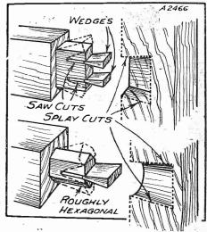
Joints made in this manner are locked into position as the two pieces of wood are fitted together.
