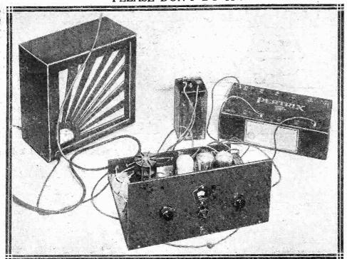
This is an excellent example of the way in which all manner of undesirable instability troubles can be produced. Never pass the loudspeaker leads under the set's baseboard, and keep them as far away from the aerial end of the set as is reasonably possible.
