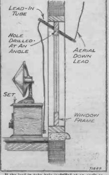
If the lead-in tube hole is drilled at an angle as illustrated above, you will have no more trouble with rain finding its way into the room.
