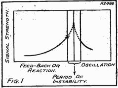
In an ordinary single-valver, working in its most sensitive condition with straightforward reaction, there is an area of instability near the point where oscillation commences. Because of this area of instability it is impossible to make the most of this reaction effect, as the set "spills over" before the boosting action attains its maximum.
