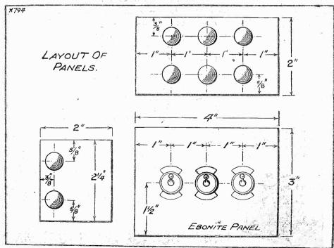
Kon will require four pieces of wood about 3 in thick, and a small piece of chonite for the panel. Although only one end and one side are shown here (those carrying the terminals) the sizes of the remaining end and side are exactly the same.
