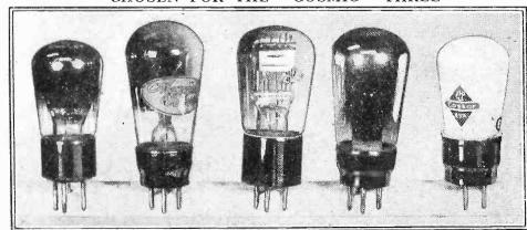
These are some more makes of valves that have been found suitable. This group contains the Mullard P.M.252, the Marconi L.2/B., Eta B.Y.2010, Mazda H.L.2, and the Cossor H.L.210. These are all 2-volt valves, and have been specially tried in the "Cosmic" circuits.
