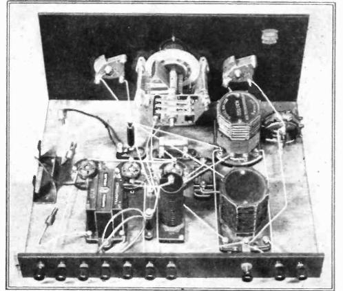
The wave-range change from medium to long waves, and vice-versa, is automatically carried out by the extenser. And by operating the little switch on the back terminal strip the set is immediately transformed into a short-waver.
