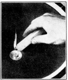
A good dodge for preventing the lock-nut of a cone loudspeaker from working loose is to seal, it in its place with a single spot of grease from a candle.
