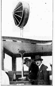
The assistant harbour-matter of the Port of London (at the wheel) with a novel soundindicator that enables ships to steer sately in fog. He got the idea from talkie technique.
