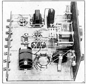
You fix the long-wave coil quoit by screwing it to a piece of wood, which in turn is held to the baseboard by another piece of wood, as shown above.
