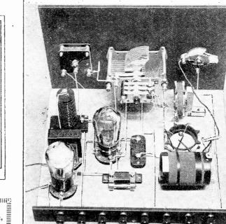
The extenser, together with a careful disposition of the components, makes the wiring particularly simple.
