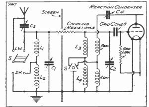
This diagram shows, in theoretical form, how the Eckersley Tuner can be connected up to an ordinary detector valve. The tuner itself includes six coil windings, the coupling resistance, and the screen. The condenser C3 is shorted out on the long waves by the double-pole switch.
