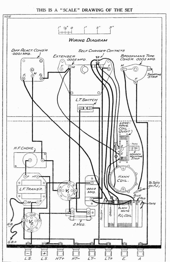
As with all "P.W." wiring diagrams, the above is drawn exactly to scale, so that you are able to place your components in exactly the same way as in the original model. The long-wave coil quoit is mounted edgewise, and is held in position by a wooden bracket (see also the photos).
