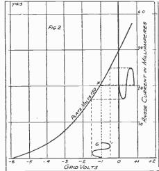
This curve shows the relation between applied grid volts and the anode current. Quite small changes of grid voltage produce tremendous swings in the plate current passing through the valve.
