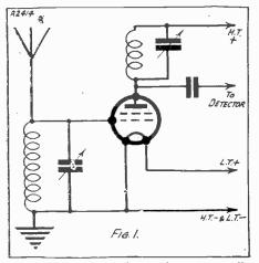
High-frequency amplification enables us to magnify the oscillations picked up by the aerial, thus greatly increasing a receiver's range. In this scheme both the grid and plate circuits of the yalve are tuned, and the amplified impulses are passed on to the detector through the fixed condenser.
