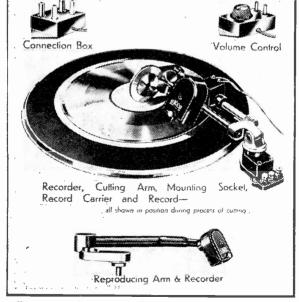
You can do all manner of things with a home recorder—record favourite radio artistes, duplicate your own records, etc. And the necessary gear is by no means complicated, as this photo of an Ekco Radiocorder clearly shows.
