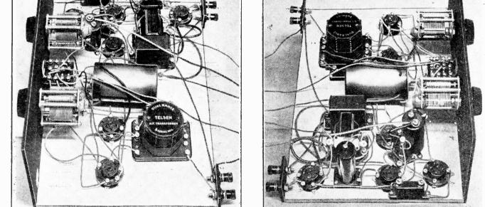
Two views of "S-Q" Star, showing its remarkable simplicity of assembly, which was enhanced still further in the final model (shown on the next pige) by the omission of the tubular condenser near the oscillator condenser.
