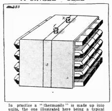
For practical purposes it matters little from what place or places the E.M.F. is derived in a thermo-electric couple; it is sufficient to know that the application of heat to one junction generates a certain E.M.F. in the circuit, the amount of which we can determine when we know 'the difference of temperature between the heated junction and the remainder of the circuit.
