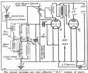
The circuit includes our very effective "P.J." system of wavechanging, which is automatically controlled by the extenser.
