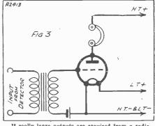
It really large outputs are required from a radio receiver, it is essential to use L.F. amplification. Part of the step-up is provided by an intervalve transformer, and the remainder by the valve.
