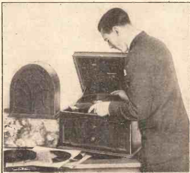
The special H.M.V. gramophone desk takes eight 10-inch or eight 12-inch records, so that you can arrange quite a pleasant little programme, put the records in place, and then leave the "works" to do the rest.
