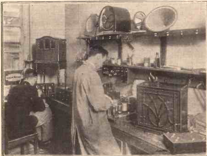
One of the main set-testing benches in "P.W.'s" Research Dept. There are duplicated high- and low-voltage points for A.C. or D.C., duplicated aerial and earth feeders connected to aerial systems of varying characteristics, and, on the top shelf, you will see a number of loudspeaker terminals with a central control switch. Below is a multi-valve output unit, giving any desired arrangement of choke or transformer output.
