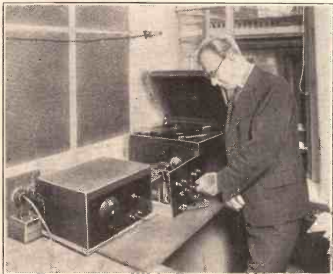
This apparatus is, in effect, a miniature broadcasting station which retains a calibrated evenness of power output and frequency stability. It is used in conjunction with a valve-voltmeter for scientifically determining the efficiencies of sets on test. Also it makes it possible to duplicate the most difficult of distant-station reception conditions, as explained in the article.
