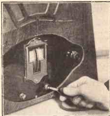
The moment the pick-up jack is inserted the set becomes an electrical record reproducer and the S.G. valve is switched out of circuit.
