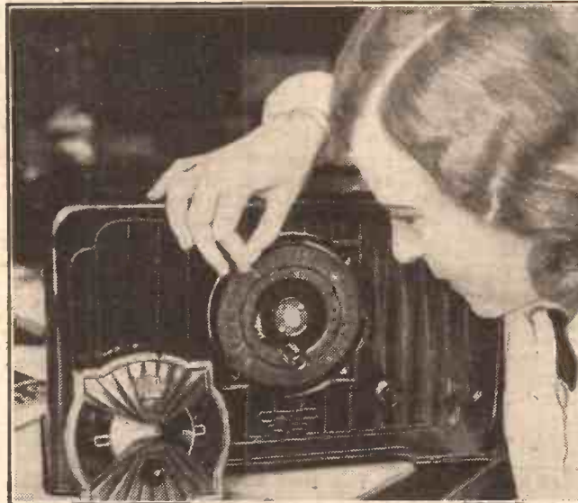
An ingenious tuning dial which was exhibited at the German Radio Show this year. It has a number of slots round its circumference in which can be inserted small tags bearing the names of broadcasting stations. In this way, once a station has been "logged," it can always be found with ease.
