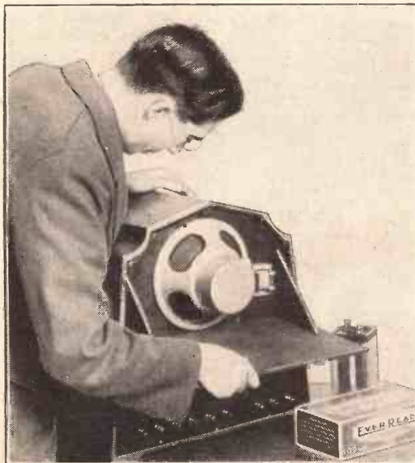
Showing how an Epoch moving-coil speaker can easily be accommodated in a "P.W." Console. The set is the Extenser "Dual-Ranger."
