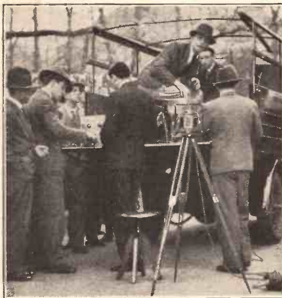
They are measuring the street noises by means of a sensitive instrument on the tripod in conjunction with the valve amplifier on the tailboard.
