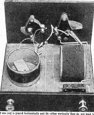
If one coil is placed horizontally and the other vertically they do not tend to "couple " and give unwanted interaction, as they would if mounted " in line,"
