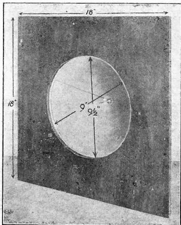
You won't find anything difficult in cutting the baffle to size. Note that the hole in it is  $\frac{1}{2}$  inch larger than the cone's diameter. This is to ensure that the edge of the cone will not touch the baffle anywhere.
