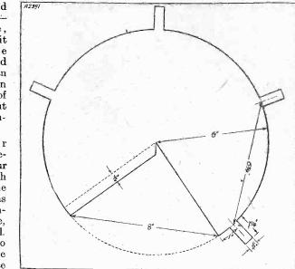
The little tabs cut as part of the cone form the mounting strips for the former, thus greatly simplifying the fixing of the cone to the baffle.
