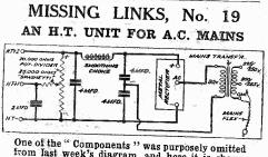
One of the "Components " was purposely omitted from last week's diagram, and here it is shown to be the smoothing choke, connected between two of the 4-mfd. condensers.
