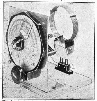
This absorption type of wave-meter consists merely of a variable condensor and a coil as shown above.
