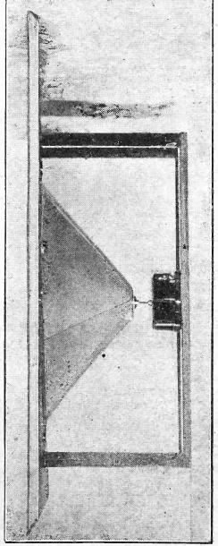
what the speaker looks like from the Note that the front edge of the cone comes flush with the back o the baffle. This is side. 1
