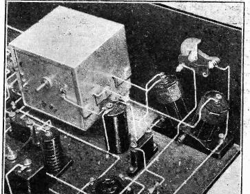
On the right and close to the panel can be seen the band-pass coil, while to the left of it is its two-gang tuning condenser.
