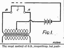
The usual method of G.B. connections, but omit-ting the secondary or other form of coupling.
