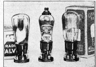
From left to right we have the Mazda AC HL, the Osram MS4B, and the Cossor M41L.F.—three notable A.C. valves.
