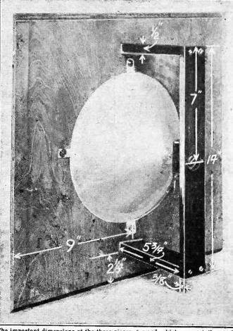
The important dimensions of the three pieces of wood which support the speaker unit are marked on this view of the back of the completed loudspeaker. The width of the three pieces is immaterial.
