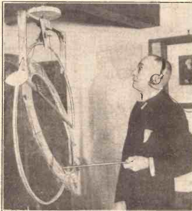
Sir Henry Jackson, Admiral of the Fleet, with an indoor aerial of his own invention. Note the nautical-looking gimbals which enable it to be rotated on an axis at any angle.
