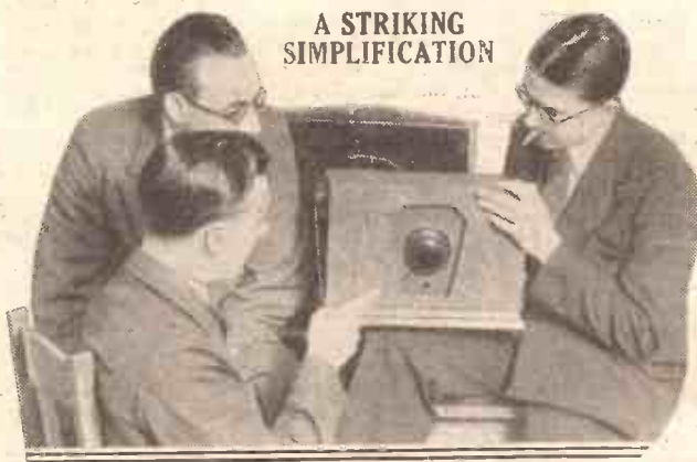
On the front there are just two controls—one to put the set on or off, and the other to tune in to all the programmes.
