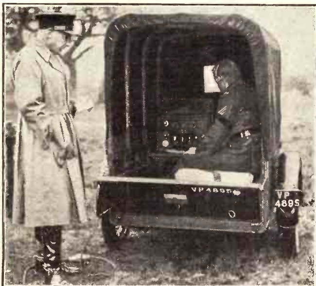
One of the new motor-cycle wireless units recently placed in commission by the 47th Divisional Signals. The special two-wheeled trailer containing a complete transmitting and receiving station is attached to a standard motor-cycle.
