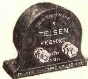
TELSEN H.F. CHOKES. Designed to cover the whole wave-band range from 1 to 4,000 metres, extremely low self-capacity, shrouded in genuine Bakelite. Inductance 150,000 microhenries. Resistance 400 ohms. Price 2/6 each.
