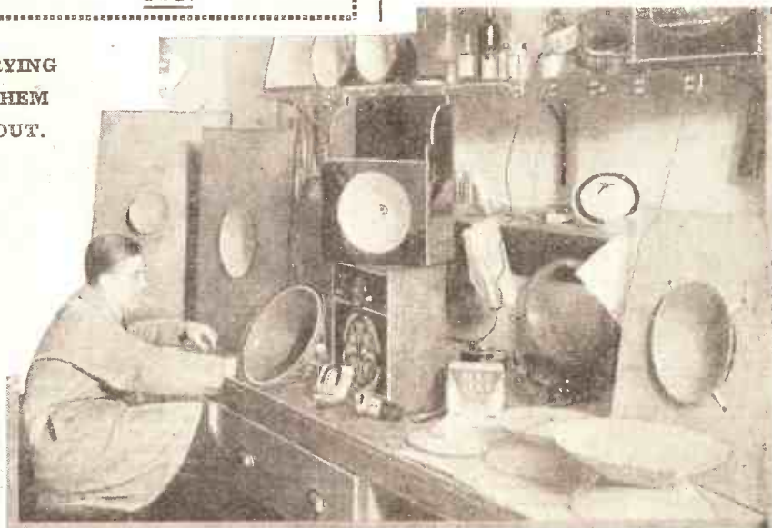
Testing out a large selection of loud speakers during stringent comparative tests carried out in connection with the trials of the new "M.W." system of "Inter-axial" suspension.
