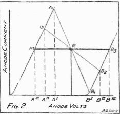
This diagram illustrates how the load-line slope varies with varying loud-speaker impedances and with varying frequencies.
