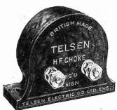
TELSEN H.F. CHOKE. D signed to cover the whole wave-band range from 18 to 4,000 metres, Extremely by week-capacity, shrouded in genuine Bakelite, Inductance 150,000 microbarries, Resistance 400 ohms.
