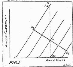
Load-lines on anode-current anode-volts curves. The full line indicates good conditions, and the dotted line bottom-bend distortion.
