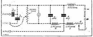
The dotted lines show the connections for the D.C. H.T. unit, the "components" for which were given last week. Note the variable voltage for H.T. + 1 (obtained by means of tapping points on the 20,000-ohms resistance) and the variable resistance R, which is of the "power" type, having a value of about 10,000 ohms.
