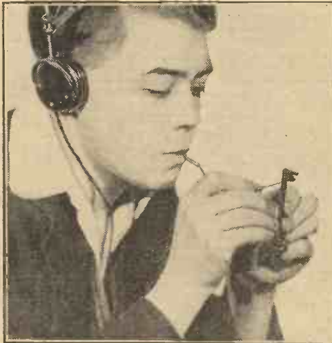
Don't test your 'phones with a dry-cell—a far more sensitive method is shown here and described on this page.
