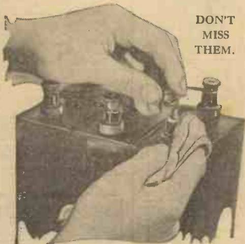
Dirty contacts in the set, leads, or batteries, will lose many a fine foreign programme, so go all-out for cleanliness.
