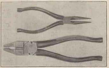
Ever tried insulated pliers? If you have to work with "live" wires sometimes they are very useful, saving the worker from shock and preventing shorts. Different kinds can be obtained, two very useful models being shown above.
