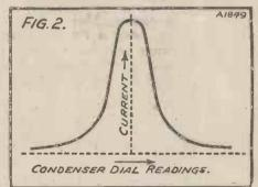
How the current in the circuit rises and falls as you go in and out of tune by varying the condenser dial position.
