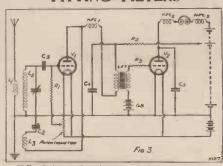
H.F. chokes and resistances used to confine the H.F. to its own parts of the circuit.
