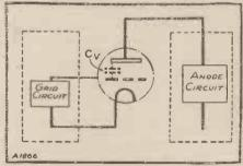
Anode and grid are coupled by the inter-electrode capacity Cv.
