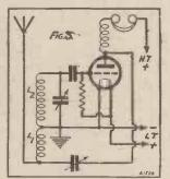
Here the extra aerial coil is eliminated, the reaction winding being made to do two jobs.
