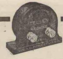
Telsen H.F. Chokes, designed to cover the whole wave-band range from 18 to 4,000 metres, extremely low self-capacity, shrouded in Genuine Bakelite. Inductance 150,000 microhenrics, resistance 400 ohms.
