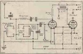
The dotted lines show how the "components" which were given in the skeleton diagram last week should be connected for a two-valver using A.C. valves.
