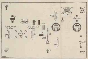
Here are the "components" for a two-valve set using indirectly-heated A.C. valves. The circuit is Detector and transformer-coupled L.F. amplifier using X-coils and a simple wave-change by means of a D.P.D.T. switch.
