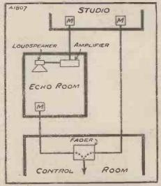
By means of a specially arranged microphone and loud speaker any amount of echo can be added to any item.
