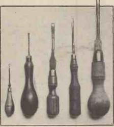
Many constructors manage with one big and one small screwdriver, but a variety of sizes for the different jobs that come along is the ideal way.
