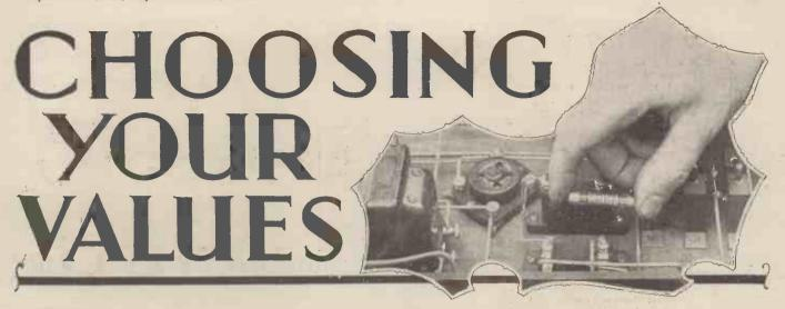
THEORETICALLY you get the greatest amplification in a given R.C.C. stage of L.F. amplification when the anode resistance is infinity. That is to say, when it has so many millions of millions of ohms that its resistance goes beyond the limits of practical measurement!
