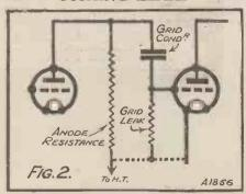
There must be a definite relation between the values of the grid condenser and grid leak if you want best results.
