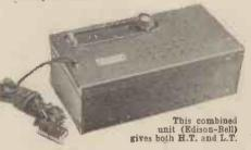
The full-wave rectifier has twisted every other half-cycle round, to line it up unidirectionally with the remainder of the current; so that in the case of fifty-cycle mains, instead of having an irregularity of 50 to work with you have a hum with a frequency of 100.
