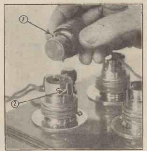
This view illustrates a simple method of ensuring that the adapter plug on the end of the twin flex lead from the accumulator always goes into its alternative sockets the right way round. Use an adapter of the wooden variety, and insert a small round-head screw exactly as you see at (1) above. Then file away a little of the metal of the holders as at (2) to admit the screw shank at one side only.
