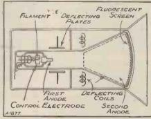
Here you can see exactly how the television cathode ray receiver is constructed. The cathode beam passes between the deflecting plates and the deflecting coils before reaching the screen.
