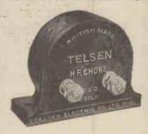
Telsen H.F. Chokes, designed to cover the whole wave-band range from 18 to 4,000 metres; extremely low self-capacity. Inductance—150,000 microhenries. Resistance—400 ohms.
