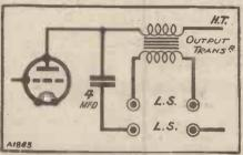
Mr. Mee used one winding of the L.F. transformer as a choke, and connected a second speaker to the other winding.
