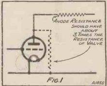
You have to take the A.C. resistance (impedance) of the valve and not its D.C. resistance.
