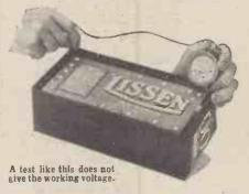
illustration, the voltage may appear much higher than it would be if the battery were supplying
