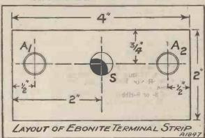
Just connect your aerial to A, and wire A, to the aerial terminal on your receiver. For work on the lower wave-band close switch S, so cutting the "Contradyne" out of circuit. Pretty easy, isn't it?
