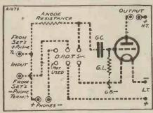
The dotted lines above indicate the connections for the amplifier, the components of which were given in last week's "Wirelet."
