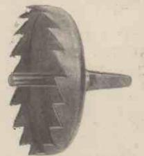
A handy device for cutting meter holes in panels.
