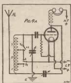
One coil only is used for long and short waves tuning, as well as for aerial coupling and reaction!
