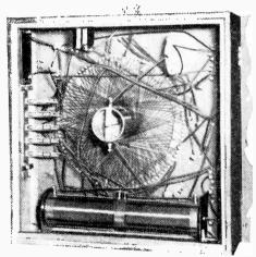
This interesting photograph shows the back view of an old crystal set made or ginally to receive the Eiffel Tower broadcasts and time signal. It measured about twenty inches square—the size of a modern portable!
