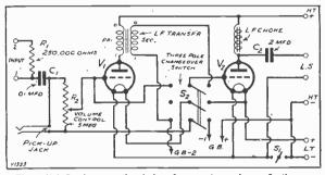
The switch  $\mathbf{S}_2$  gives you the choice of one or two valves. In the one valve position it also turns off the filament of the unused valve.
