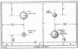
The panel lay-out is perfectly symmetrical, so you can do your marking out on the back without troubling about right and left.
