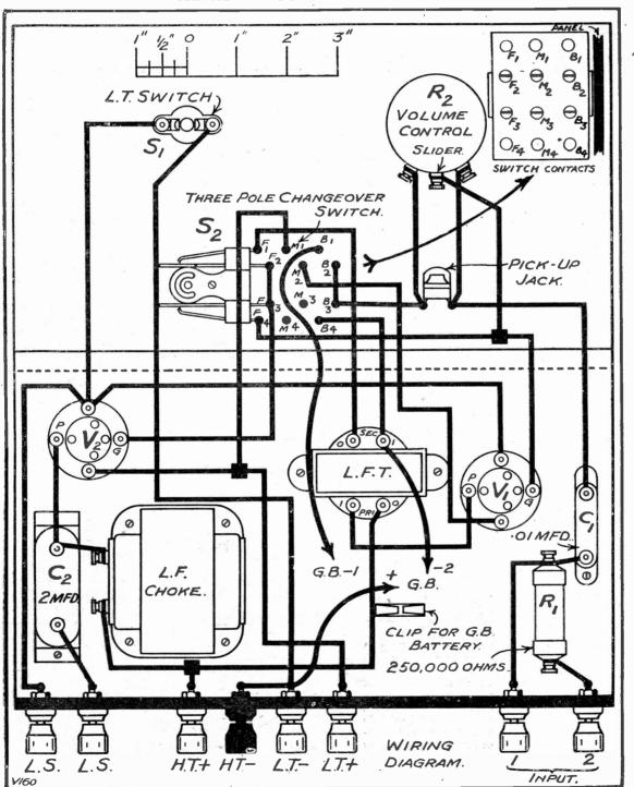
The wiring is easy enough to carry out, but just a little care is needed in making the connections to S, and checking them up. There is a key to the positions of the various contacts in one corner of this diagram which you will find makes everything quite plain when you bave the switch before you. The H.T. negative terminal is marked in black to emphasise an important point which is explained in the text.
