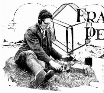
THE current produced in a frame acrial depends on the difference between the effect of the wave upon one vertical side of the frame and that upon the other vertical side of the frame at the same moment. It will be clear from this that if the frame is placed "broadside on" to the waves, the effect on the two vertical sides of the frame at any instant will be the same, that is, the difference will be zero, and therefore there will not be any electromotive force induced in the frame.
