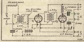
Here are the connections of last week's two-valve amplifier, shown by the dotted lines. It can be used with a crystal or small valve set and will give great power and purity, with the advantages of volume control and choke-filtered output.
