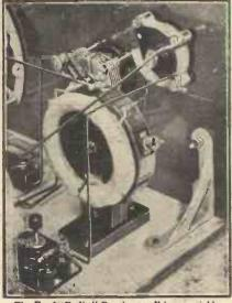
The Ready Radio "Brookmans" type variable condenser seen at the top right-hand corner is extremely convenient for fitting into receivers where space is limited.
