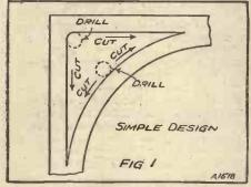
Saw cuts should always be made towards sharp corners, as even a fretsaw will give a rounded effect which looks "amateurish."
