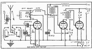
you ever .cen such a simple wave-change circuit as Remember that it uses plug-in coils and absolutely standard parts.
