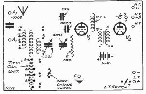
Here are all the necessary "components" for a two-valve set (Det. and L.F.) with a "Titan" tuner for wave-change. The 0001 reaction condenser has a 001 fixed condenser in series with it, to prevent shorting, and the circuit is otherwise perfectly straightforward. Could you wire it up?
